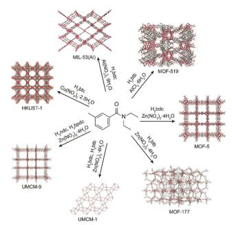
Fig. 3 Metal-organic frameworks successfully synthesized in DEET along with their precursor metal salts and linker acids
