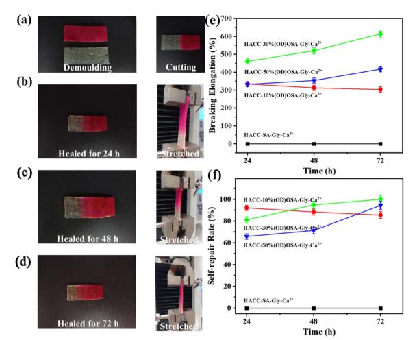
Fig. 6 (a)–(d) Self-healing process and tensile test of the HACC-50%(OD)OSA-Gly-Ca<sup>2+</sup> hydrogel after self-healing; (e) elongation of four kinds of hydrogels after a period (72 h) of self-healing; (f) self-repair rate of four kinds of hydrogels after a period (72 h) of self-healing
