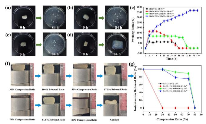
Fig. 7 (a) HACC-SA-Gly- $Ca^{2+}$ , (b) HACC-10%(OD)OSA-Gly- $Ca^{2+}$ , (c) HACC-30%(OD)OSA-Gly- $Ca^{2+}$ , and (d) HACC-50%(OD)OSA-Gly- $Ca^{2+}$  dry gels were soaked for 84 h, respectively; (e) swelling rate curves of the four kinds of hydrogels; (f) the process of HACC-50%(OD)OSA-Gly- $Ca^{2+}$  hydrogel compression experiment; (g) variation of compressive rebound of the four kinds of hydrogels.
