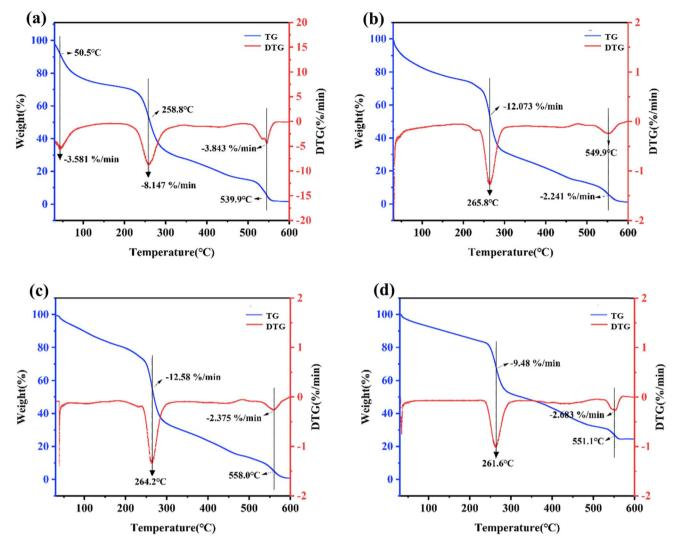
Fig. 4 TG and DTG curves of the four different kinds of hydrogels: (a) HACC-SA-Gly-Ca $^{2+}$ ; (b) HACC-10%(OD)OSA-Gly-Ca $^{2+}$ ; (c) HACC-30%(OD)OSA-Gly-Ca $^{2+}$ ; (d) HACC-50%(OD)OSA-Gly-Ca $^{2+}$ .
