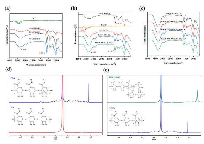
Fig. 2 (a-c) FTIR spectra of (a) SA, 10%(OD)OSA, 30%(OD)OSA, and 50%(OD)OSA; (b) hydrogels of 50(OD)%OSA, HACC, HACC, HACC-50%(OD)OSA, HACC-50%(OD)OSA-Gly-Ca<sup>2+</sup>; (c) and the self-healing hydrogels of HACC-SA-Gly-Ca<sup>2+</sup>, HACC-10%(OD)OSA-Gly-Ca<sup>2+</sup>, HACC-10%(OD
