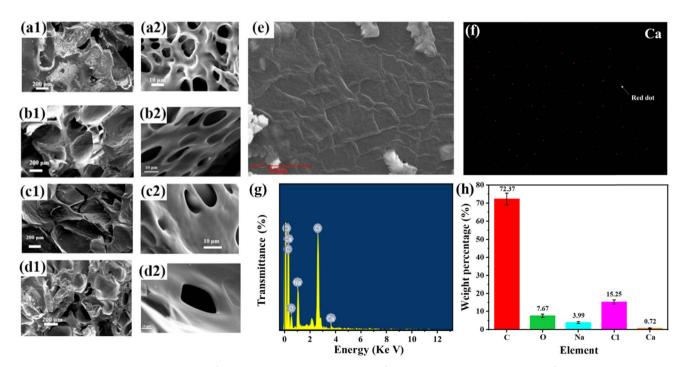
Fig. 3 SEM images of (a) HACC-SA-Gly-Ca<sup>2+</sup>, (b) HACC-10%(OD)OSA-Gly-Ca<sup>2+</sup>, (c) HACC-30%(OD)OSA-Gly-Ca<sup>2+</sup>, and (d) HACC-50%(OD)OSA-Gly-Ca<sup>2+</sup> hydrogels; (e) SEM image with local magnification of  $8000 \times$  of the HACC-50%(OD)OSA-Gly-Ca<sup>2+</sup> hydrogel; (f) calcium distribution, indicated by red dot; (g) EDS analysis diagram of HACC-50%(OD)OSA-Gly-Ca<sup>2+</sup> hydrogel; (h) elemental quantitative analysis.
