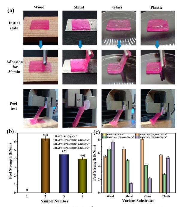
Fig. 8 Adhesion and stripping behaviors of HACC-50%(OD)OSA-Gly-Ca<sup>2+</sup> hydrogels on wood, steel, plastic, and glass; (b) average peel strength of the four kinds of hydrogels on various substrates; (c) peel strength of the four kinds of hydrogels on various substrates.
