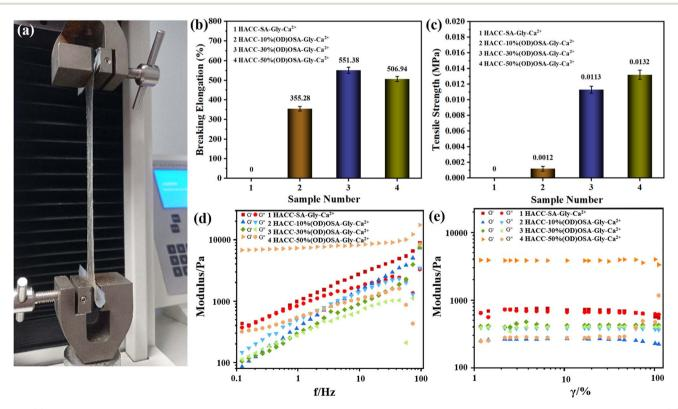
Fig. 5 (a) Test setup using the electronic universal tensile testing machine to test the mechanical properties of the four types of hydrogel: (b) elongation at break; (c) tensile strength; (d) curves of the energy storage modulus (G') and loss modulus (G') with the change of frequency; (e) curves of the energy storage modulus (G') and loss modulus (G') with the change of strain.
