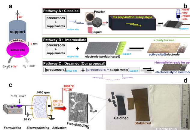
**Fig. 1** (a) The “support-contact-active-site” model of the electrocatalyst. (b) The three approaches to the fabrication of a catalytic electrode. (c) The design methodology that combines the electrospinning and two thermal treatments.
