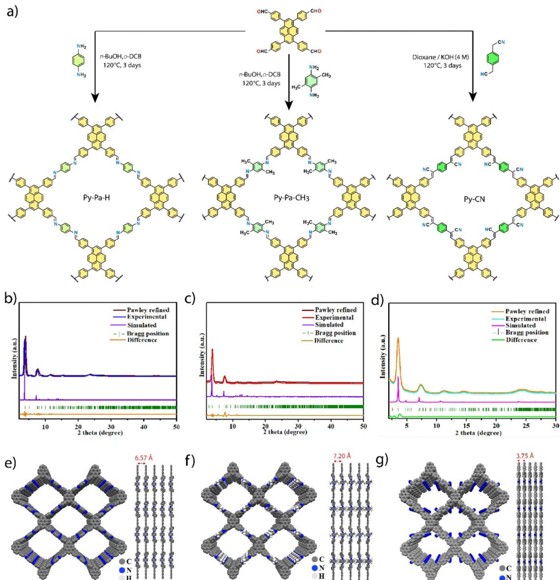
**Fig. 1** Synthesis of pyrene-based donor–acceptor COFs. (a) Scheme of the synthesis of Py-Pa-H, Py-Pa-CH<sub>3</sub> and Py-CN COFs. Comparison of simulated and experimental PXRD patterns for (b) Py-Pa-H, (c) Py-Pa-CH<sub>3</sub> and (d) Py-CN COFs. The ideal AA eclipsed (AA) stacking mode for (e) Py-Pa-H, (f) Py-Pa-CH<sub>3</sub>, and (g) Py-CN COFs.
