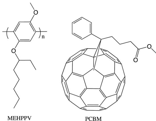
Fig. 3 The structures of MEHPPV and PCBM.
