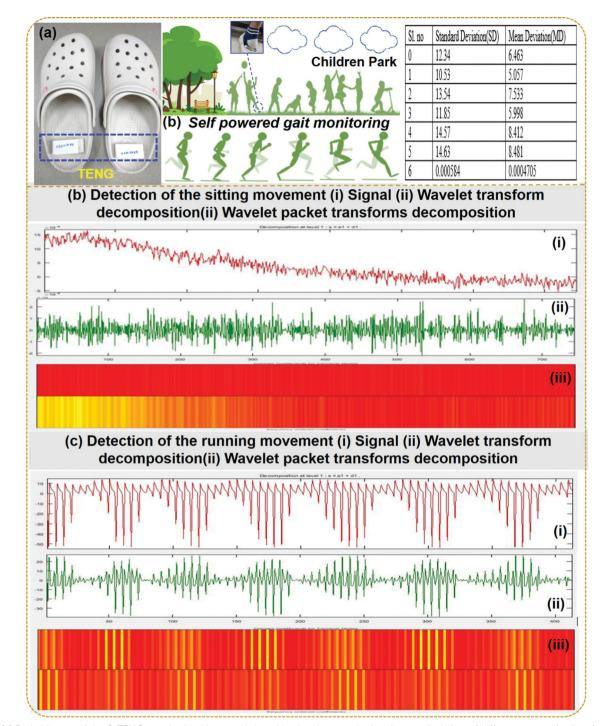
Fig. 6 (a) Digital image of the S-TENG attached to shoes and the table showing standard and mean deviation of different types of gaits of volunteers; (b) detection of the sitting signal: (i) signal from the S-TENG device while sitting, (ii) wavelet transform decomposition, and (iii) wavelet packet transform decomposition; (c) detection of the running movement: (i) signal from the S-TENG device while running, (ii) wavelet transform decomposition, and (iii) wavelet packet transform decomposition.
