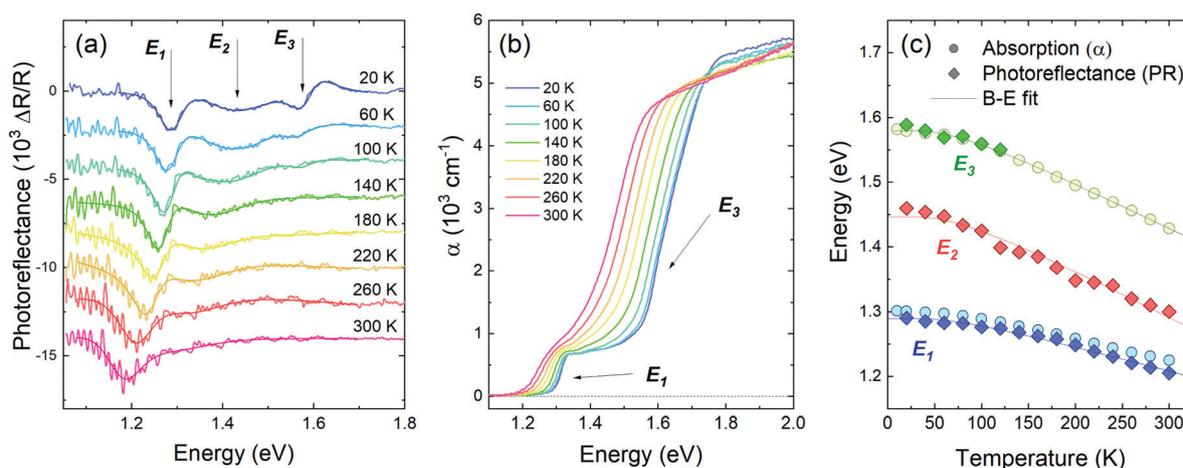
Fig. 3 Photoreflectance (a) and optical absorption (b) spectra measured at different temperatures from 20 to 300 K, and the temperature dependence of the optical transition energies observed in PR (diamond symbols) and absorption (circles), fitted with the Bose–Einstein formula given by eqn (3) (solid lines) (c).
