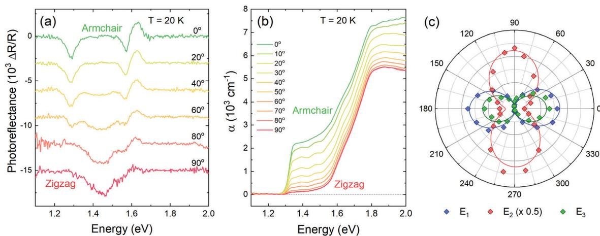
**Fig. 4** Photorefectance (a) and optical absorption (b) spectra acquired for light polarized linearly from 0° (along the armchair crystallographic direction) to 90° (along the zigzag direction). Polarization dependence of transition oscillator strength, calculated as the integrated area under the PR resonance modulus curve (c).
