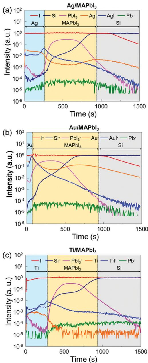
Fig. 4 ToF-SIMS depth profiles of (a) the Ag/MAPbI<sub>3</sub>, (b) the Au/MAPbI<sub>3</sub>, and (c) the Ti/MAPbI<sub>3</sub> stacks.
