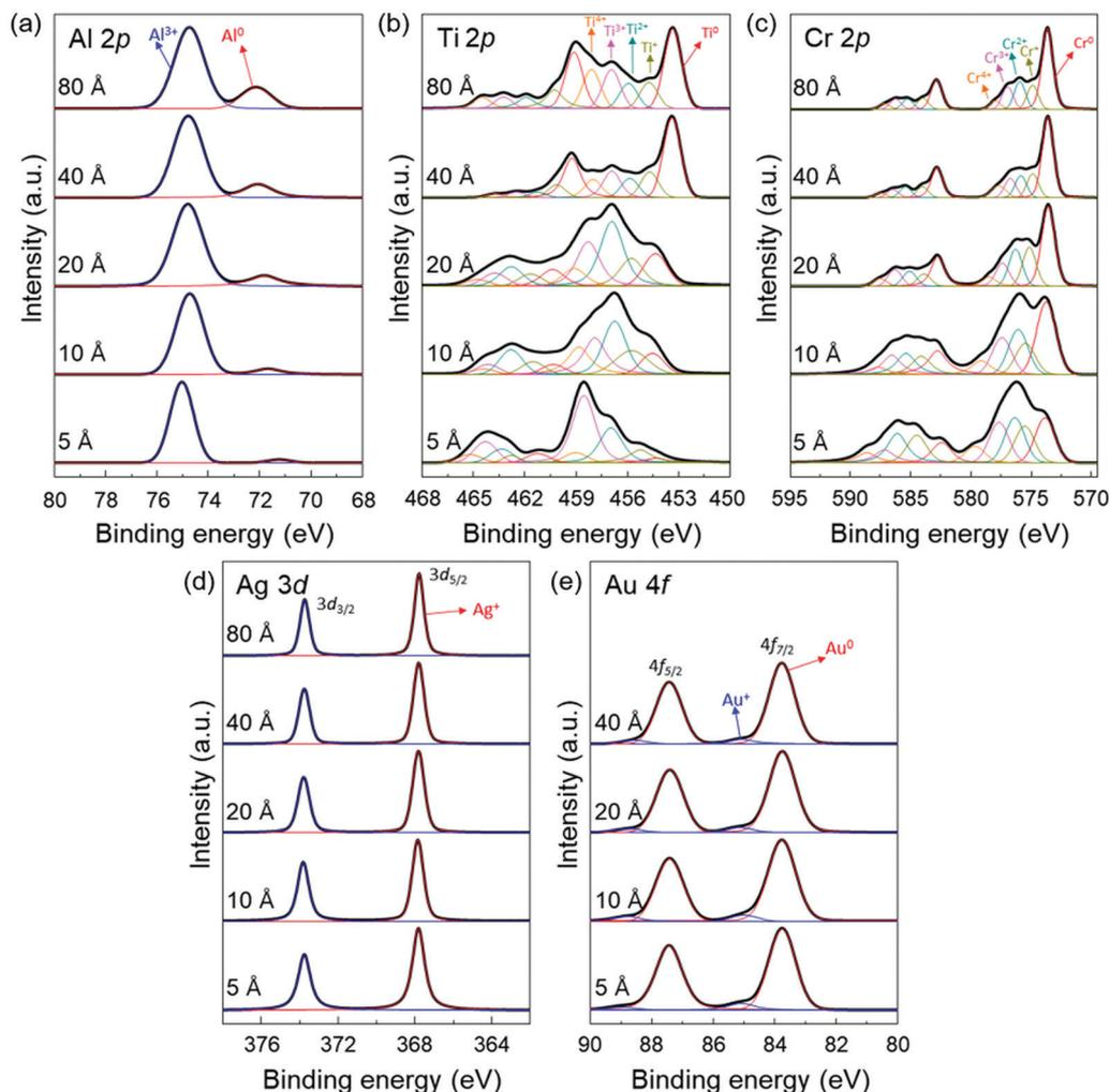
Fig. 3 Thickness dependent XPS spectra of (a) the Al 2p peaks in the Al/MAPbI<sub>3</sub> thin films, (b) the Ti 2p peaks in the Ti/MAPbI<sub>3</sub> thin films, (c) the Cr 2p peaks in the Cr/MAPbI<sub>3</sub> thin films, (d) the Ag 3d peaks in the Ag/MAPbI<sub>3</sub> thin films, and (e) the Au 4f peaks in the Au/MAPbI<sub>3</sub> thin films.
