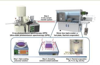
Scheme 1 Schematic illustration for preparation and characterization process of metal/MAPbI<sub>3</sub> thin films.
