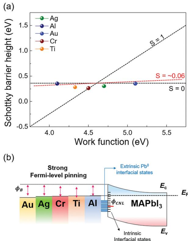
Fig. 5 (a) Extracted Schottky barrier heights of MAPbI<sub>3</sub> for the various metal work functions, showing the pinning factor  $S \sim 0.06$  when the deposited metal thickness is 40 Å (red dashed line). (b) Band diagram of metal/MAPbI<sub>3</sub> interfaces with five different metals.
