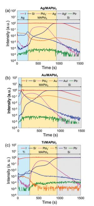
Fig. 4 ToF-SIMS depth profiles of (a) the Ag/MAPbl<sub>3</sub>, (b) the Au/MAPbl<sub>3</sub>, and (c) the Ti/MAPbl<sub>3</sub> stacks
