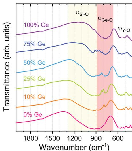
Fig. 2 FTIR spectra of the  $Y_2(Ge_xSi_{1-x})O_5:Pr$  materials.
