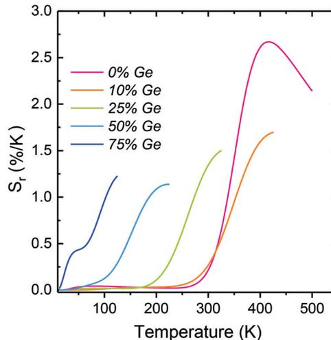
Fig. 7 Relative thermal sensitivity ( $S_r$ ) based on the 5d → 4f decay traces of the Y<sub>2</sub>(Ge<sub>*x*</sub>Si<sub>1-*x*</sub>)O<sub>5</sub>:Pr materials.
