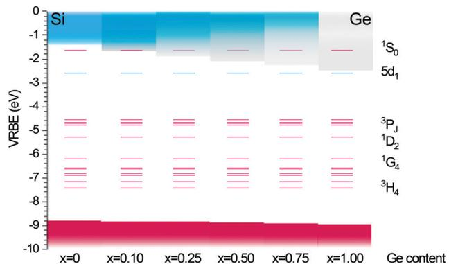
Fig. 1 The effect of the Ge:Si ratio on the bandgap structure of the Y<sub>2</sub>(Ge<sub>x</sub>Si<sub>1-x</sub>)O<sub>5</sub> host lattices and the relative position of the electronic levels of Pr<sup>3+</sup>.
