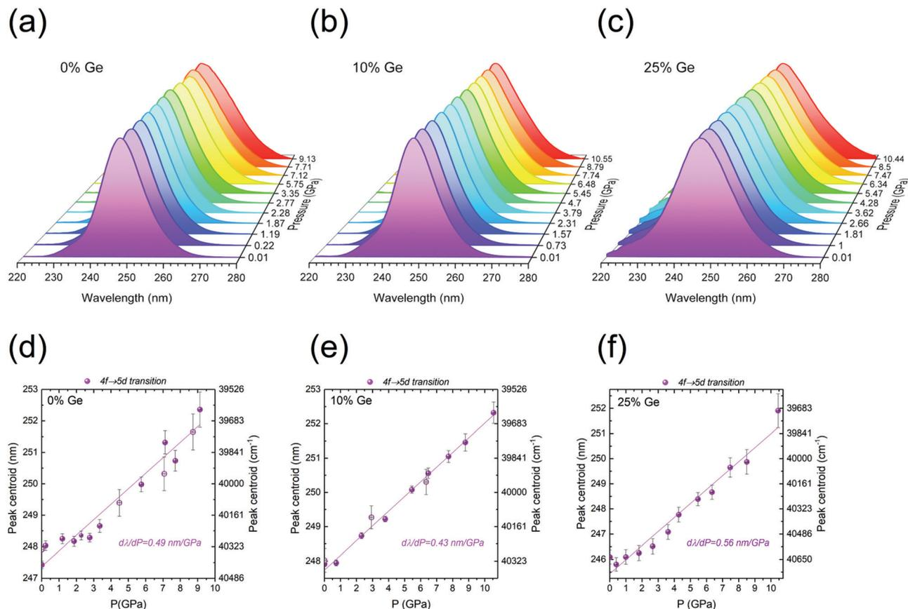
Fig. 9 Normalized PLE spectra of the  $Y_2(Ge_xSi_{1-x})O_5:Pr$  samples with 320 nm luminescence as a function of pressure, where  $x =$  (a) 0, (b) 0.10, and (c) 0.25 of Ge. Spectral positions of the  $4f \rightarrow 5d$  excitation band for the  $Y_2(Ge_xSi_{1-x})O_5:Pr$  samples, where  $x =$  (d) 0, (e) 0.10, and (f) 0.25.
