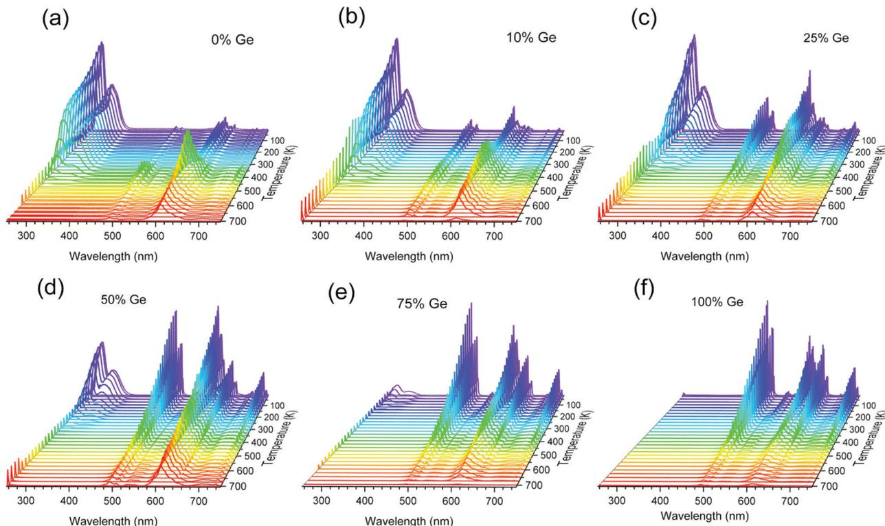
Fig. 4 Temperature-dependent photoluminescence spectra of the  $Y_2Ge_xSi_{1-x}O_5:0.05\%Pr$  phosphors, in the  $T$ -range of 11–700 K. (a)  $x = 0$ , (b)  $x = 0.10$ , (c)  $x = 0.25$ , (d)  $x = 0.50$ , (e)  $x = 0.75$ , and (f)  $x = 1.0$ .
