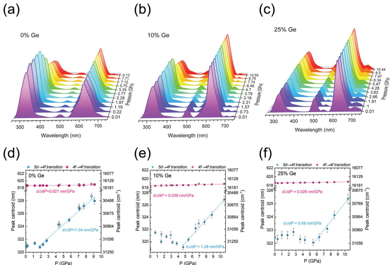
Fig. 8 PL emission spectra of the  $Y_2(Ge_xSi_{1-x})O_5:Pr^{3+}$ , where  $x =$  (a) 0, (b) 0.10, and (c) 0.25 ( $\lambda_{ex} = 248$  nm), measured as a function of pressure, in the range of 0–10 GPa. The determined spectral positions of the  $Pr^{3+}$   $4f \rightarrow 4f$  (red) and  $5d \rightarrow 4f$  (blue) emission bands, as a function of pressure for 0, 0.10, and 0.25 of Ge are presented in (d)–(f), respectively.
