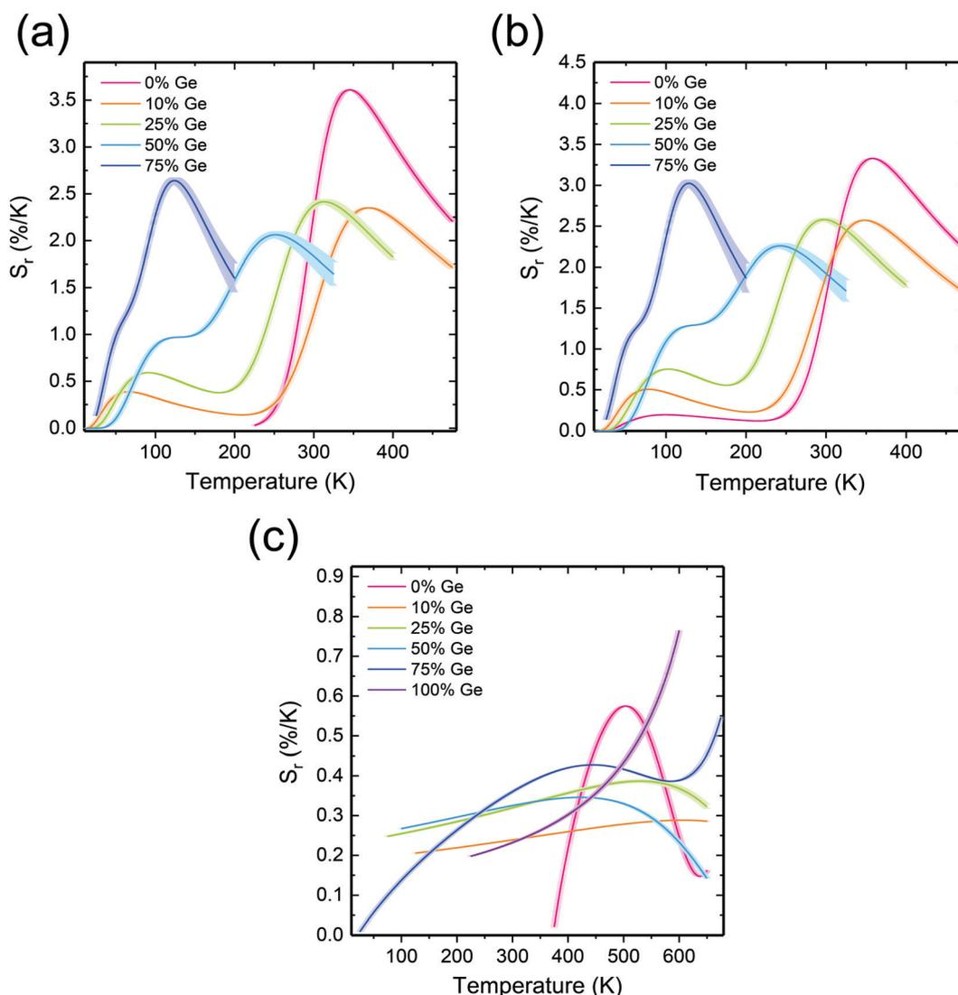
Fig. 6 Temperature dependence of the relative thermal sensitivity (eqn (4)) based on (a) LIR<sub>1</sub>, (b) LIR<sub>2</sub>, and (c) LIR<sub>3</sub>.
