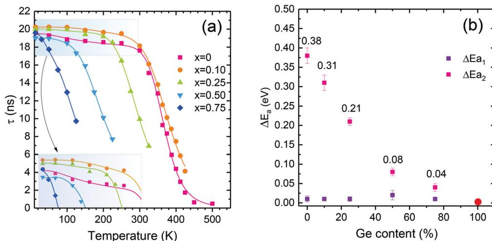
Fig. 5 (a) Temperature dependence of the  $5d \rightarrow 4f$  PL decay time of the  $Y_2(Ge_xSi_{1-x})O_5:Pr$  phosphors, under 250 nm excitation. The inset is a magnification of the low-temperature range of the curves to better reveal the complex shape of the curves in the low range of temperature. (b) Dependence of the activation energies,  $\Delta E_{a1}$  and  $\Delta E_{a2}$ , of the  $5d \rightarrow 4f$  emission thermal quenching, derived using eqn (1).
