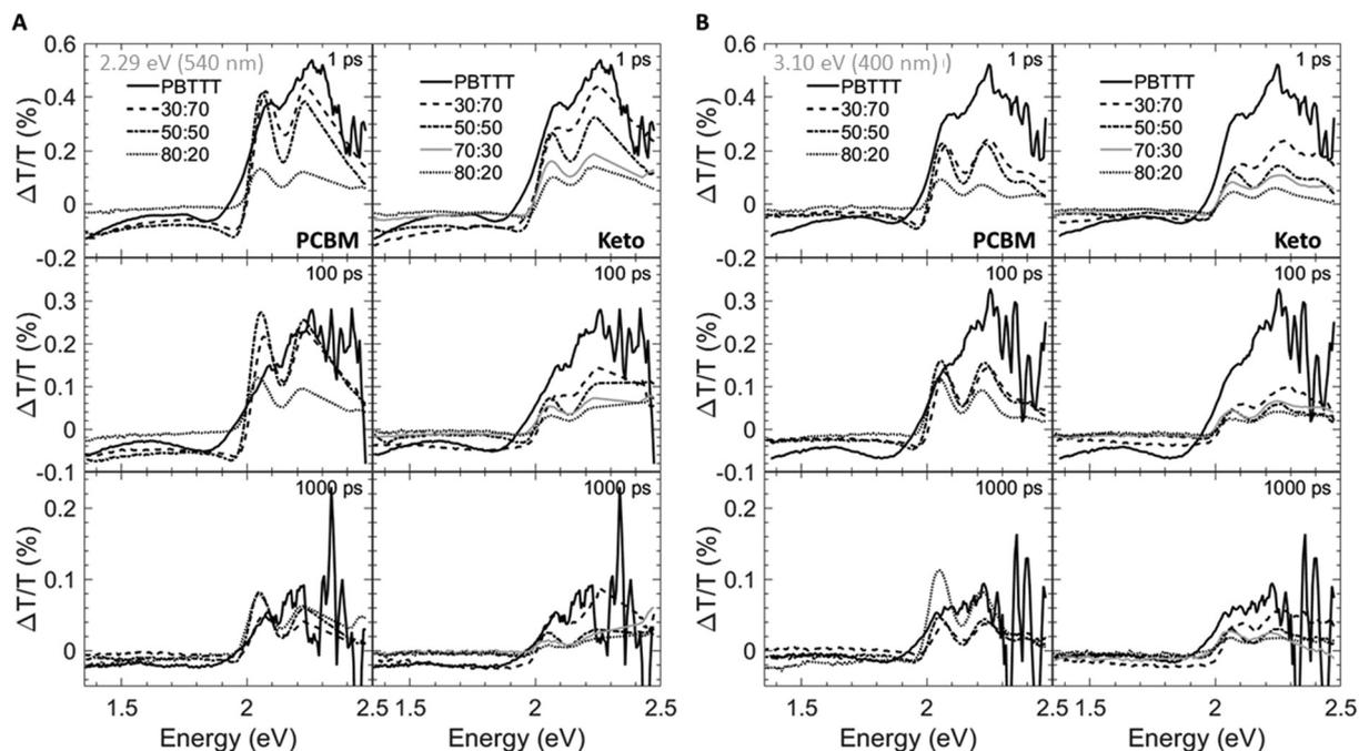
Fig. 4 Spectral transient-absorption cuts taken at different delay times (1 ps: top panels; 100 ps: middle panels; 1000 ps: bottom panels) for fullerene:**PBTBT** blends photoexcited at 2.29 eV (540 nm) (A) and 3.1 eV (400 nm) (B). Data for **PCBM**-based binaries are shown in the left panels; those for **ketolactam** systems on the right.
