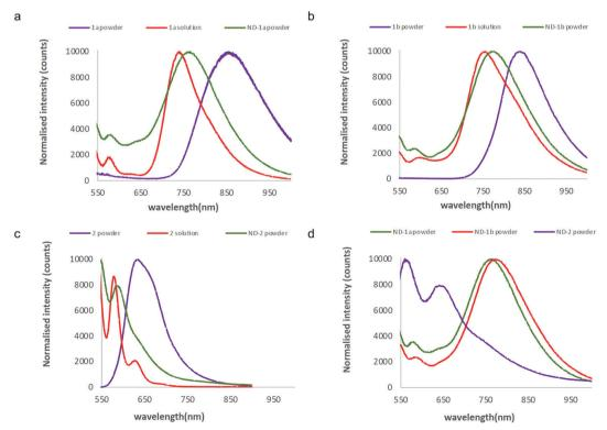
Fig. 3 Normalised fluorescence spectra comparing the different ND-PDIs (green), parent PDI in solid-state (purple) and in chloroform solution (red). (a) ND-1a/1a; (b) ND-1b/1b; and (c) ND-2/2. (d) Comparison of spectra for ND-1a (green), ND-1b (blue), ND-2 (purple).
