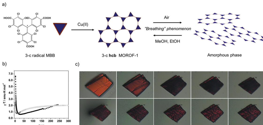
**Fig. 4** (a) Schematic representation of the formation of **hcb** MOROF-1 using the 3-c PTMTC and Cu(II), and its breathing behaviour. (b) Value of  $\chi T$  as a function of the temperature for MOROF-1 (filled circle, MOROF-1; open circle, evacuated and amorphous MOROF-1 phase). (c) Breathing phenomenon of a single crystal of MOROF-1 when exposed to the air (top) and re-exposed to ethanol liquid (bottom). (b and c) Adapted from ref. 69. Copyright 2003 Nature Group.
