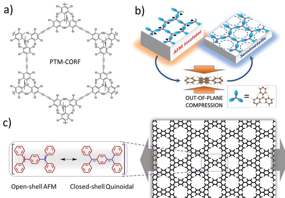
**Fig. 5** (a) Synthesised PTM-CORF. Adapted from ref. 78. Copyright 2018 Wiley-VCH Verlag GmbH & Co. (b) Mott-like transition in a ring-sharing hexagonal 2D CORF upon out-of-plane pressure. Reprinted from ref. 80. Copyright 2021 Wiley-VCH Verlag GmbH & Co. (c) Transition between open-shell AFM state and closed-shell quinoidal state in a ring-sharing 2D CORF induced by in-plane strain. Reprinted from ref. 84. Copyright 2021 Nature Group.
