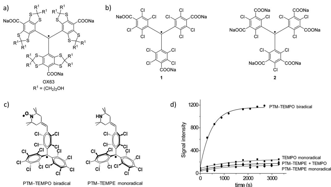
Fig. 8 (a) OX63. (b) Two different PTM derivatives functionalized with three (1) and six (2) carboxylate groups.<sup>124</sup> (c) Molecular structures of biradical PTM-TEMPO and monoradical PTM-TEMPE. (d) Polarization building curves (3.35 T, 1.4 K) of biradical PTM-TEMPO (90 mM) at 94.067 GHz, monoradical PTM-TEMPE (90 mM) at 94.08 GHz, 4-oxo-TEMPO (90 mM) at 94.120 GHz, and a mixture of monoradical PTM-TEMPE and 4-oxo-TEMPO both at 90 mM.<sup>116</sup>
