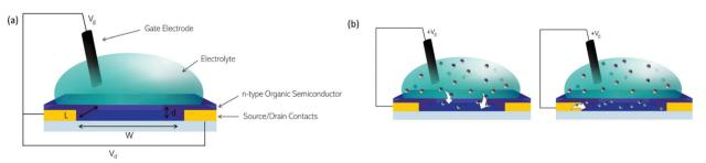
Fig. 13 (a) Architecture of an OECT. (b) Illustrations of (left) migration of positive ions from aqueous electrolyte into an n-type organic semiconductor on application of a positive gate bias. (right) Compensation of positive charges in the organic semiconductor film by electrons.
