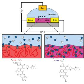
Fig. 14 The molecular structures of the all alkyl OTFT material (P-0) and all glycol OECT material (P-100) and schematic illustrations of their operation. Cations are depicted in blue, anions in white and electrons throughout the polymer backbone are grey. Adapted from literature. 80,142
