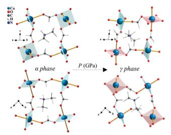
Fig. 1 Crystal structure of the  $\alpha$ -phase at ambient pressure and  $\gamma$ -phase at 9.1 GPa. The equatorial planes are drawn in blue and red. JT axis are shown as yellow sticks.
