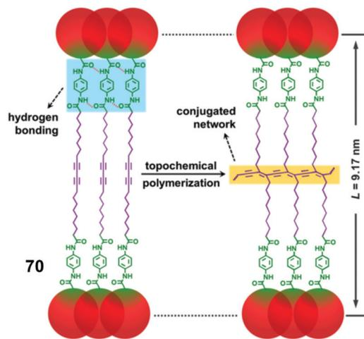
Fig. 26 Molecular packing of self-assembled butadiynyl derivative **70** before and after photopolymerisation. The red circles represent dendron units. Reproduced from ref. 184 with permission from the Royal Society of Chemistry.
