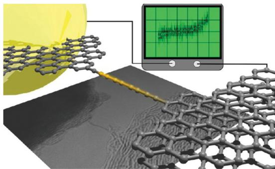
Fig. 12 Schematic representation and TEM image of a conducting monoatomic carbon chain between graphene electrodes and an  $I$ - $V$  trace of the device. Reproduced from ref. 125 with permission from the American Chemical Society.
