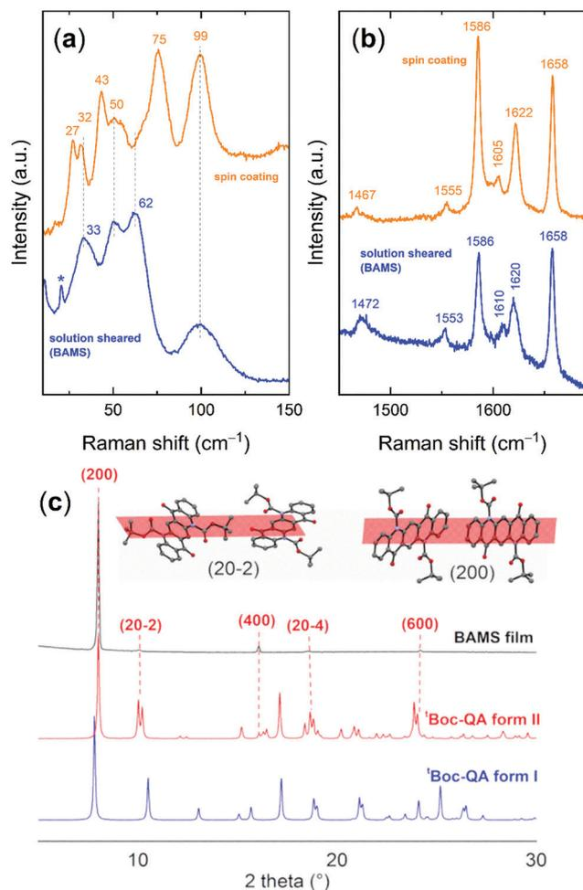
**Fig. 6** (a) Lattice phonon and (b) intramolecular Raman spectra of spin cast and BAMS  $\beta$ Boc-QA films; (c) diffraction patterns of BAMS films and the two  $\beta$ Boc-QA polymorphs. Inset: Orientation of the two  $\beta$ Boc-QA molecules with respect of the (20-2) and (200) Miller planes in form II. H<sub>CH</sub> atoms omitted for clarity.
