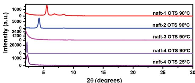
Fig. 10  $\theta$ – $2\theta$  X-ray diffraction scans of vapor-deposited **naft-1–4** thin films ( $T_d = 25^\circ \text{C}$  and  $90^\circ \text{C}$ ) grown on OTS-treated Si/SiO<sub>2</sub> substrates.
