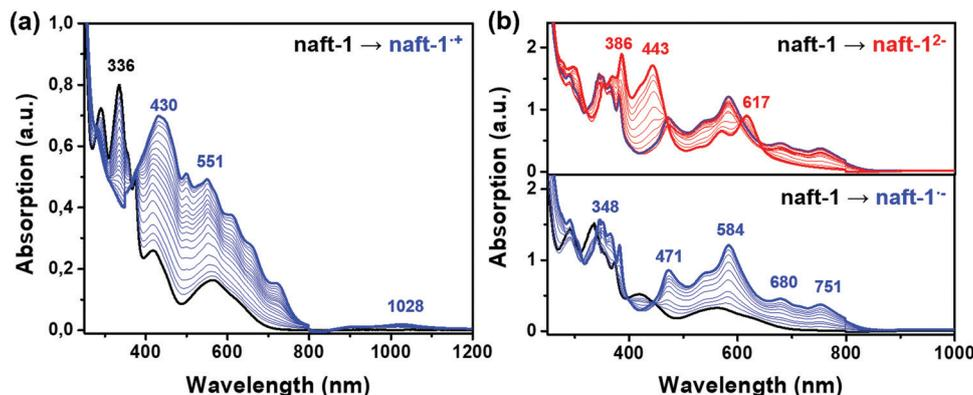
**Fig. 7** UV-Vis-NIR absorption spectra recorded in an OTTE cell by (a) electrochemical oxidation (1520 mV, blue curve), (b) during the first step of electrochemical reduction ( $-790$  mV, blue curve) and during the second step of the electrochemical reduction ( $-1040$  mV, red curve) of **naft-1** in dichloromethane in presence of  $\text{Bu}_4\text{NBF}_4$  supporting electrolyte.
