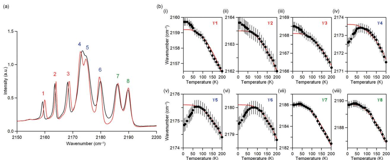
Fig. 3 Temperature dependence of the IR spectrum of MnW. (a) IR spectrum at 5 K (red) and 60 K (black). (b) IR peak frequency due to the CN stretching mode,  $\nu_i$  ( $i = 1\text{--}8$ ), vs. temperature plots. Red line indicates the peak position obtained by fitting the theoretical equation of thermal expansion<sup>61</sup> due to anharmonic phonons without magnetic ordering. Error bars indicate the resolution of the apparatus.
