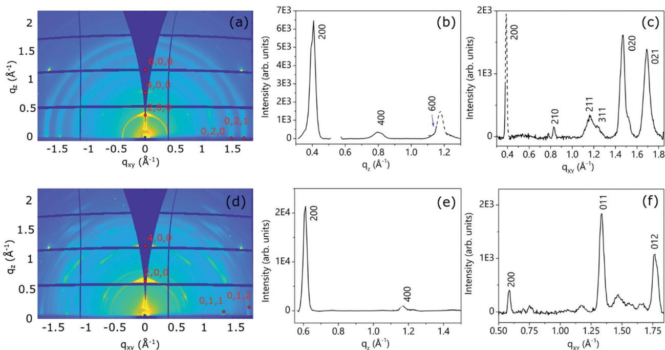
Fig. 9 2D-GIXD images of annealed (a) NmpDI and (d) NphDI thin films recorded for  $\alpha_i = 0.1^\circ$ . The corresponding integrated intensity profiles along  $q_z$ , [(b) and (e)], and along  $q_{xy}$ , [(c) and (f)] are reported. The dashed lines in b, c and e are Gaussian fits to the experimental data at the positions where the detector cuts hamper collection of the diffracted intensity.
