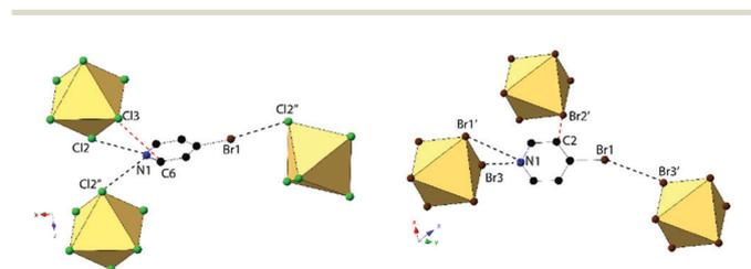
Fig. 6 Local structure of **3** (left) and **7** (right) showing hydrogen and halogen bonding (black dashed lines). Short X··C contacts shown as red dashed lines. Compound **7** assumes a different packing scheme and space group (*P1* vs. *P2(1)/c*) from compound **3**.
