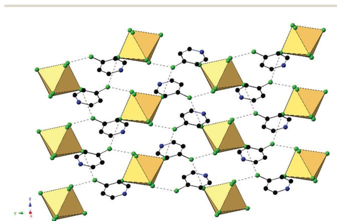
Fig. 5 Packing of **2** highlighting the extended halogen bonding (dashed lines) between [TeCl<sub>6</sub>]<sup>2-</sup> octahedra and associated ClPy cations.
