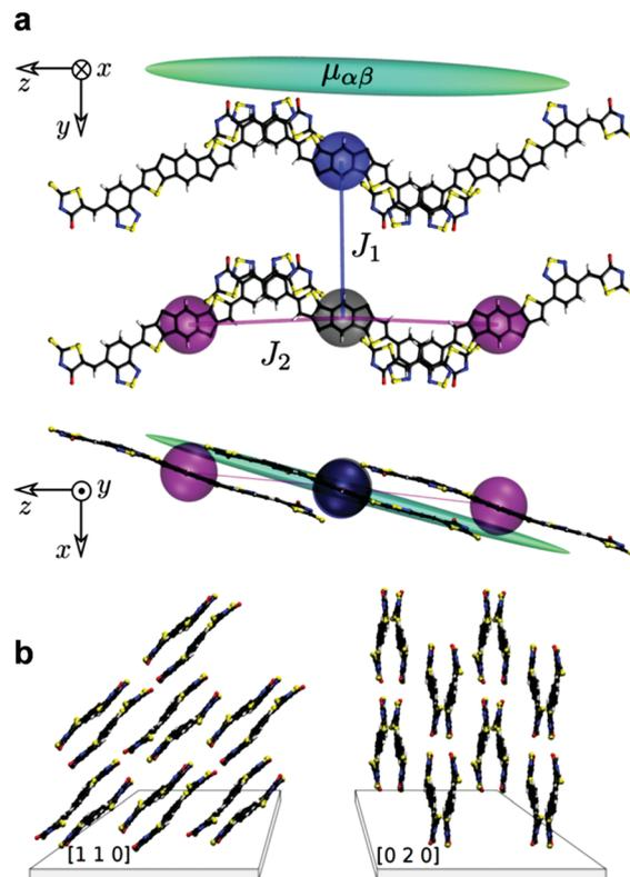
Fig. 5 (a) Packing of O-IDTBR (side chains are omitted) with spheres showing the geometrical centers of molecules. Lines show charge hopping directions, with electronic couplings  $J_2 \sim 2J_1$ . Mobility tensor  $\hat{\mu}$  is visualized by an ellipsoid and is very anisotropic due to orientation of the preferential orientation of long molecular axes along the  $z$ -direction. (b) The [110] and [020] orientations of the unit cell with respect to the substrate.
