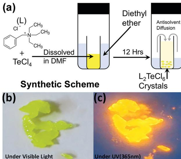
Fig. 1 (a) Reaction scheme (anti-solvent diffusion) utilized for the synthesis of single crystals of  $(\text{BzTEA})_2\text{TeCl}_6$ ; photograph of the synthesized crystals at room temperature under (b) visible and (c) UV illumination (365 nm).
