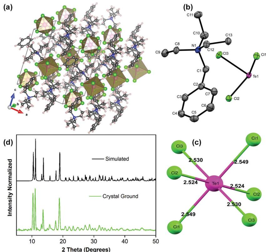
Fig. 3 XRD characterization of the  $(\text{BzTEA})_2\text{TeCl}_6$  hybrid. Overview of the single crystal structure (a); asymmetric unit (b); site symmetry of Metal-Halide octahedron (c); comparison of the simulated and experimental PXRD pattern using Cu source (d). H atoms are omitted in (b) for clarity.
