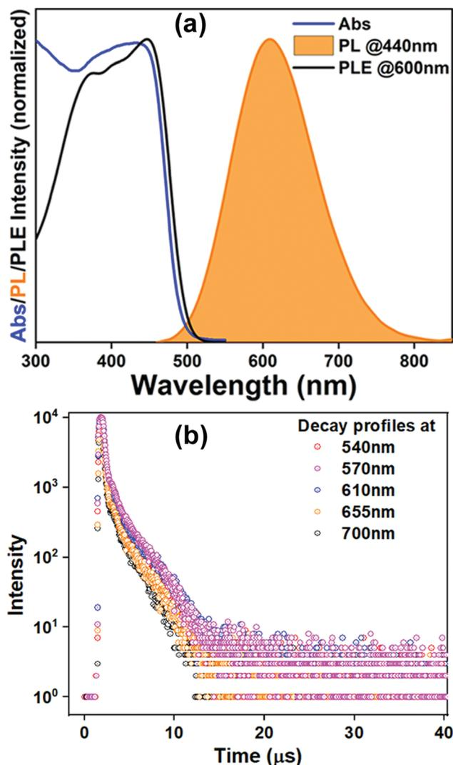
Fig. 2 Optical characterization of  $(\text{BzTEA})_2\text{TeCl}_6$  showing (a) absorbance (Abs), photoluminescence (PL), and photoluminescence excitation (PLE) spectra; (b) lifetime decay profiles collected across the PL band ( $\lambda_{\text{exc}} = 440$  nm).
