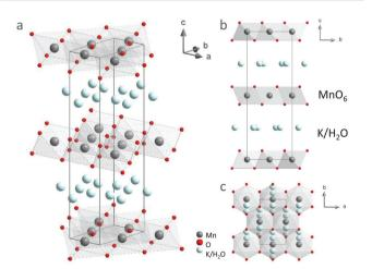
Fig. 5 Schematic representation of the crystal structure of  $\rm K_{0.31}MnO_2\cdot 0.41H_2O$ . The manganese and oxygen atoms are represented by dark grey and red spheres respectively; the potassium atoms and the  $\rm H_2O$  molecules are represented by light blue spheres. One unit cell is indicated by the dark grey lines.
