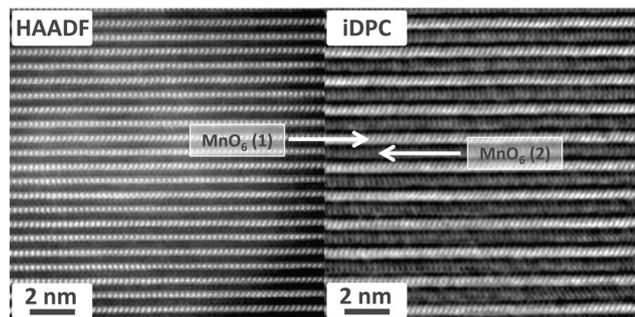
Fig. 8 iDPC-STEM image (right) of a representative nanodomain shows alternating contrast of the  $\text{MnO}_6$  planes due to charge ordering of  $\text{Mn}^{3+}/\text{Mn}^{4+}$ , which is not seen in the HAADF-STEM image (left).
