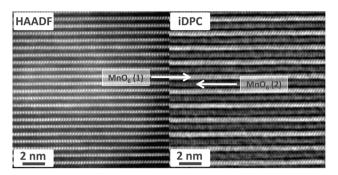
Fig. 8 iDPC-STEM image (right) of a representative nanodomain shows alternating contrast of the  $MnO_6$  planes due to charge ordering of  $Mn^{3+}/Mn^{4+}$ , which is not seen in the HAADF-STEM image (left).
