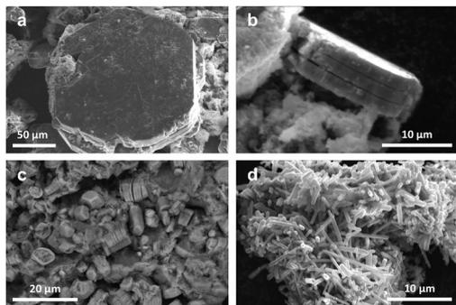
Fig. 1 SEM images of (a) K-bir single crystal grown using  $\text{KNO}_3\text{--B}_2\text{O}_3$  flux and alumina crucible (sample 1) viewed perpendicular to  $a\text{--}b$  plane and (b) perpendicular to  $c$ -axis; (c) sample synthesized using  $\text{KNO}_3\text{--B}_2\text{O}_3$  flux and Pt crucible (sample 2); (d) sample synthesized with  $\text{PbO--B}_2\text{O}_3$  flux and Pt crucible (sample 3).
