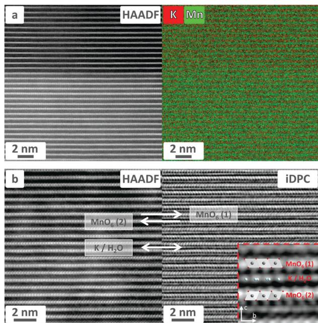
Fig. 6 (a) HAADF-STEM image of K-bir and corresponding EDS map showing Mn and K planes perpendicular to  $c$ -axis; (b) HAADF-STEM image of K-bir and corresponding iDPC-STEM imaging revealing the existence of two layers of  $\text{MnO}_6$  octahedra with opposite tilt angles, separated by layers of K atoms and  $\text{H}_2\text{O}$  molecules.
