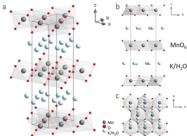
Fig. 5 Schematic representation of the crystal structure of  $K_{0.31}MnO_2 \cdot 0.41H_2O$ . The manganese and oxygen atoms are represented by dark grey and red spheres respectively; the potassium atoms and the  $H_2O$  molecules are represented by light blue spheres. One unit cell is indicated by the dark grey lines.
