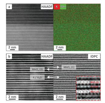
Fig. 6 (a) HAADF-STEM image of K-bir and corresponding EDS map showing Mn and K planes perpendicular to c-axis; (b) HAADF-STEM image of K-bir and corresponding iDPC-STEM imaging revealing the existence of two layers of MnO<sub>6</sub> octahedra with opposite tilt angles, separated by layers of K atoms and H<sub>2</sub>O molecules.
