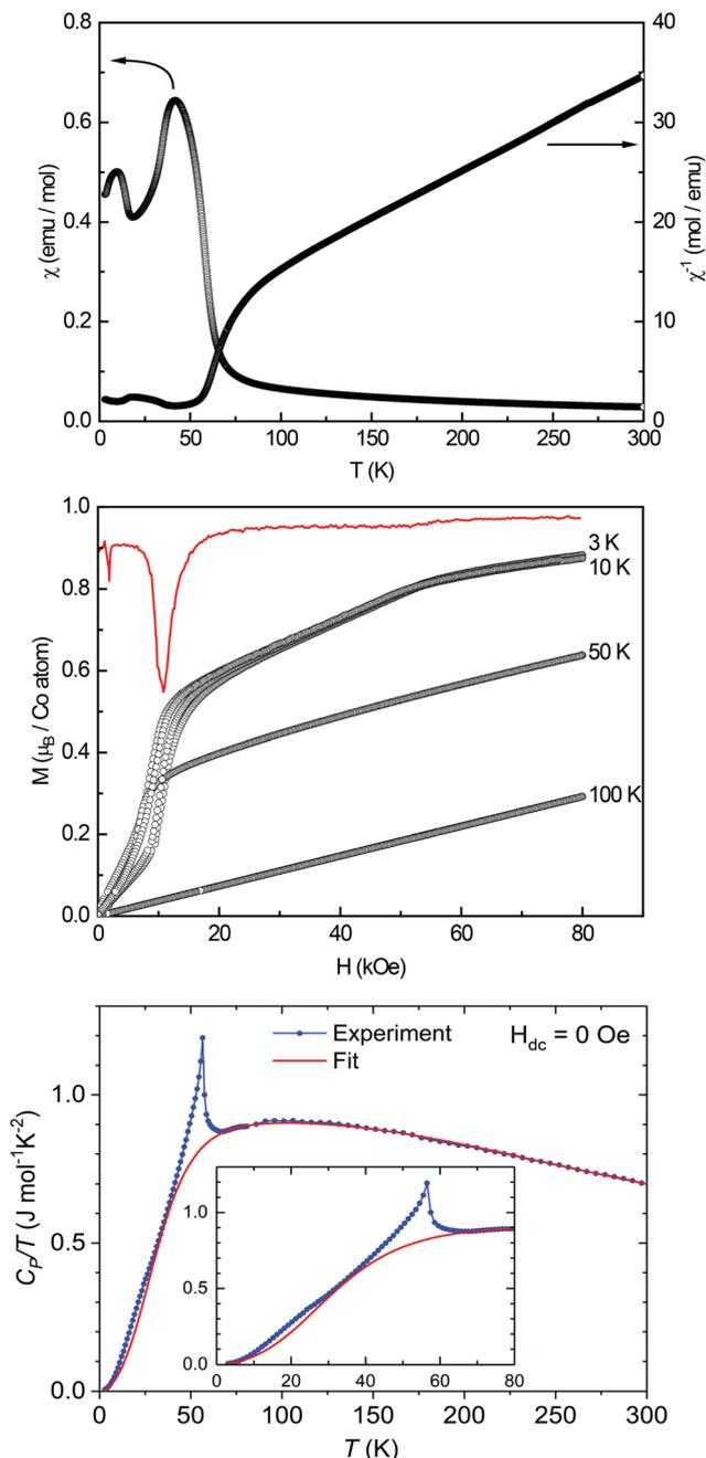
Fig. 6 Magnetic properties of HP-Co<sub>3</sub>TeO<sub>6</sub>: susceptibility and inverse susceptibility ( $\chi$  and  $\chi^{-1}$ ), measured in an external field strength of 10 kOe (top); magnetization isotherms recorded at 3, 10, and 50 K, the derivative  $dM/dH$  is depicted in red (middle); temperature dependence of  $C_p/T$  of HP-Co<sub>3</sub>TeO<sub>6</sub> at zero field (blue line and circles) with the corresponding Einstein–Debye fit (red line) (bottom).
