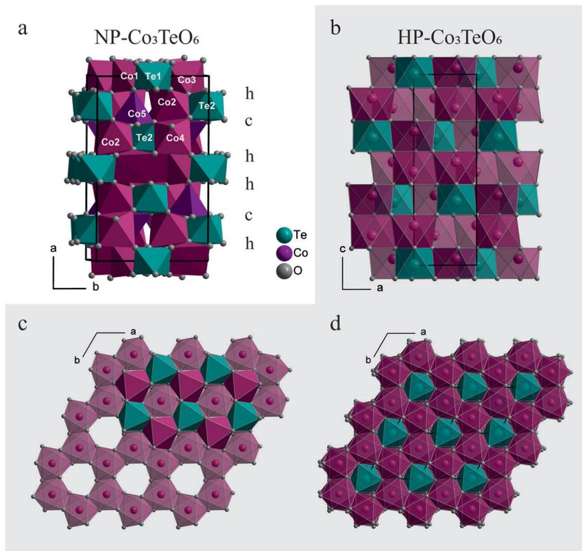
Fig. 2 The crystal structure of NP- $\text{Co}_3\text{TeO}_6$  is shown in (a). The five different Co coordination polyhedra are marked. The crystal structure of HP- $\text{Co}_3\text{TeO}_6$  with a view along the  $b$ -axis and view along the  $c$ -axis are given in (b) and (d), respectively.  $\text{TeO}_6$ - and  $\text{CoO}_6$ -octahedra are drawn in violet and teal. (c) Illustrates the stacking of the honeycomb-ordered layers along the  $c$ -axis.
