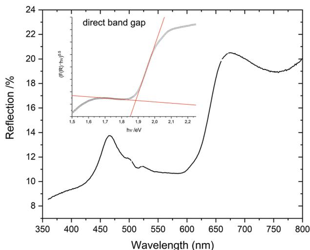
Fig. 5 UV-Vis reflectance spectra of HP-Co<sub>3</sub>TeO<sub>6</sub> and Tauc plot (inset) assuming a direct band gap.
