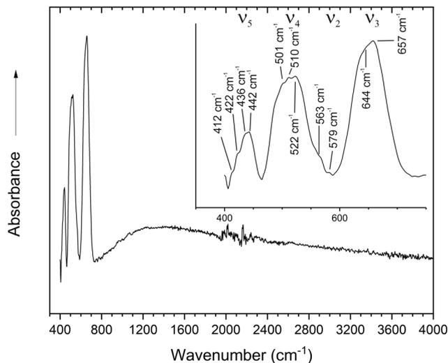
Fig. 4 FT-IR-spectra of HP-Co<sub>3</sub>TeO<sub>6</sub>.
