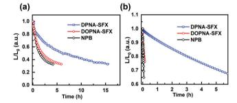
Fig. 6 Normalized luminance as a function of operating time for (a) red and (b) green PHOLEDs with different HTMs
