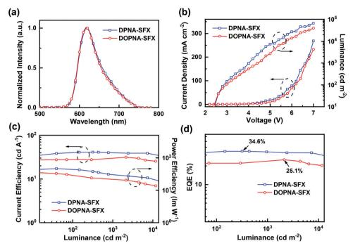
Device performance of red PHOLEDs: (a) EL spectra (4.0 V), (b) J-V-L curves, (c) CE-L-PE curves, and (d) EQE-L curves
