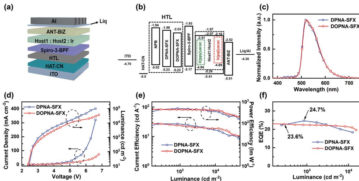
Fig. 3 (a) Device architecture of PHOLEDs and (b) energy diagram of multilayer PHOLEDs. Device performances of green PHOLEDs: (c) EL spectra (4.0 V), (d)  $J$ - $V$ - $L$  curves, (e) CE- $L$ -PE curves, and (f) EQE- $L$  curves.
