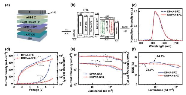
Fig. 3 (a) Device architecture of PHOLEDs and (b) energy diagram of multilayer PHOLEDs. Device performances of green PHOLEDs: (c) EL spectra (4.0 V), (e) J–V–L curves, (f) CE–L–PE curves, and (g) EQE–L curves.
