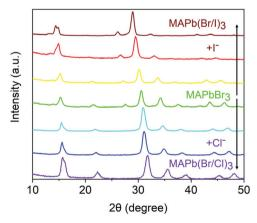
Fig. 2 Powder X-ray diffraction (XRD) patterns of the synthesized MAPbX<sub>3</sub> films.
