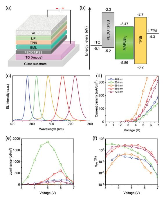
Fig. 4 EL characteristics using our synthesized anion exchanged MAPbX<sub>3</sub> perovskite NCs. (a) Schematic device architecture. (b) Schematic energy level diagram based on the parent MAPbBr<sub>3</sub> NCs. (c) EL spectra of the fabricated LEDs. Characterized (d) current density, (e) luminance, and (f) external quantum efficiency as a function of voltage.
