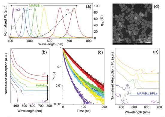
Fig. 3 Normalized (a) PL and (b) absorption spectra of the parent MAPbBr<sub>3</sub> and mixed-halide perovskite NCs together with their  $\eta_{PL}$ . (c) Time-resolved photoluminescence (TRPL) responses of the synthesized NCs. (d) Representative transmission electron micrograph of 2D MAPbBr<sub>3</sub> NPLs (scale bar: 50 nm). (e) Absorption (solid lines) and PL (dashed lines) of the LASPS synthesized mixed-halide perovskite NPLs.
