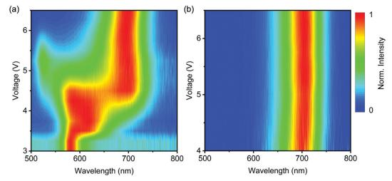
Fig. 5 EL spectra of KI-exchanged MAPb(Br/I)<sub>3</sub> under electrical stress. (a) The evolution of EL spectra as a function of driving voltage. (b) EL spectra of the color-stable mixed-halide MAPb(Br/I)<sub>3</sub> NCs after applying a reverse bias of -4 V for 20 minutes.
