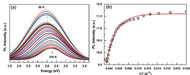
Fig. 3 (a) Temperature-dependent PL spectra of OA-capped  $\text{Cs}_3\text{BiBr}_6$  NCs at the temperature range of 50–300 K. (b) Integrated PL intensity of  $\text{Cs}_3\text{BiBr}_6$  NCs versus inverse temperature and the Arrhenius fitting.
