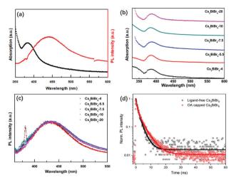
Fig. 2 Optical properties for ligand-free Cs<sub>3</sub>BiBr<sub>6</sub> NCs: (a) absorption spectra and PL spectra for Cs<sub>3</sub>BiBr<sub>6</sub>-5.5 NCs. (b) Absorption spectra for different ratios of precursors. (c) PL spectra for the addition of different ratios of precursors. (d) TR-PL kinetics of Cs<sub>3</sub>BiBr<sub>6</sub>-5.5 NCs with and without OA capping measured with TCSPC (375 nm pump) fitted with a bi-exponential function
