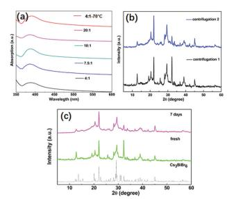
Fig. 4 Stability for  $Cs_3BiBr_6$  ligand-free NCs. (a) UV-vis absorption spectra after wash treatment with IPA twice. (b) XRD pattern after washing treatment by IPA twice. (c) XRD patterns for fresh and aged samples after 7 days.
