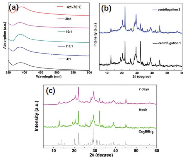
Fig. 4 Stability for  $\text{Cs}_3\text{BiBr}_6$  ligand-free NCs. (a) UV-vis absorption spectra after wash treatment with IPA twice. (b) XRD pattern after washing treatment by IPA twice. (c) XRD patterns for fresh and aged samples after 7 days.
