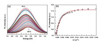
Fig. 3 (a) Temperature-dependent PL spectra of OA-capped Cs<sub>3</sub>BiBr<sub>6</sub> NCs at the temperature range of 50-300 K. (b) Integrated PL intensity of Cs<sub>3</sub>BiBr<sub>6</sub> NCs versus inverse temperature and the Arrhenius fitting
