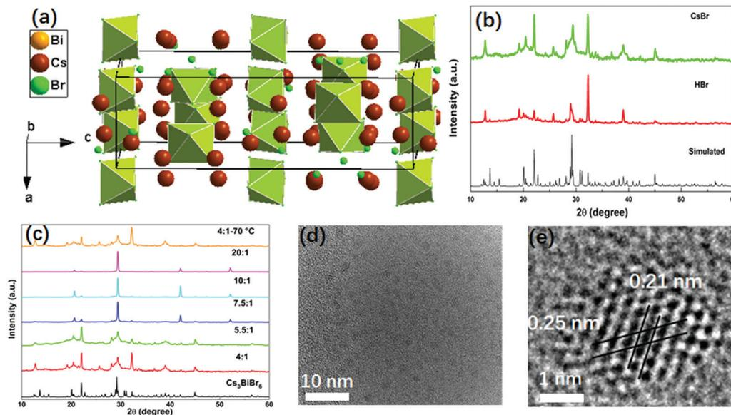
Fig. 1 (a) Crystal structure of  $\text{Cs}_3\text{BiBr}_6$ . (b) XRD pattern of  $\text{Cs}_3\text{BiBr}_6$  NCs with addition of CsBr or HBr precursors and the simulated XRD pattern (CCDC, #1877001). (c) XRD pattern of  $\text{Cs}_3\text{BiBr}_6$  for several precursor ratios of CsBr/BiBr<sub>3</sub> at room temperature and at 70 °C. (d) Representative TEM image for  $\text{Cs}_3\text{BiBr}_6$ -5.5 NCs. (e) HRTEM image with an atomic resolution for a  $\text{Cs}_3\text{BiBr}_6$ -5.5 NC.
