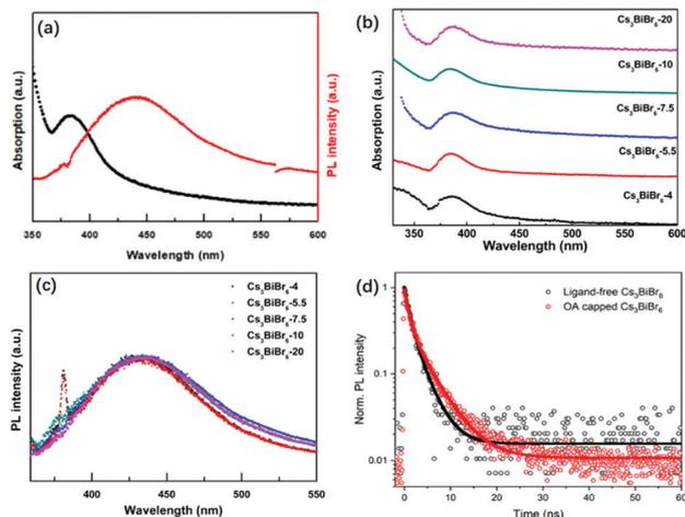
Fig. 2 Optical properties for ligand-free  $\text{Cs}_3\text{BiBr}_6$  NCs: (a) absorption spectra and PL spectra for  $\text{Cs}_3\text{BiBr}_6$ -5.5 NCs. (b) Absorption spectra for different ratios of precursors. (c) PL spectra for the addition of different ratios of precursors. (d) TR-PL kinetics of  $\text{Cs}_3\text{BiBr}_6$ -5.5 NCs with and without OA capping measured with TCSPC (375 nm pump) fitted with a bi-exponential function.
