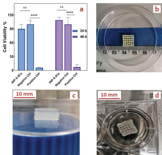
Fig. 7 (a) Comparison of cell viability at 24, and 48 h in the extract of ink 3NF-0.5Ca via SRB assay. (Two-way ANOVA, Sidak's post-test,  $p < 0.0001$ ). The lattice-structure printed scaffolds: (b) scaffolds after printing and before photo crosslinking, (c) photo crosslinked scaffolds after swelling in culture media for 48 h, and (d) scaffolds with fibroblasts seeded on top after 1 week in culture media.
