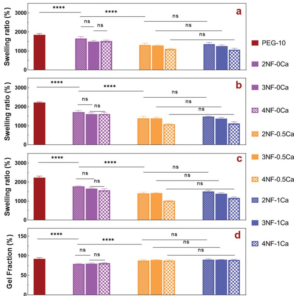
Fig. 5 Water uptake of different PEG-CNF hydrogel inks. Equilibrium mass swelling ratios of PEG-CNF hydrogels formed with various contents of CNFs or  $\text{Ca}^{2+}$  ( $n = 5$ , mean  $\pm$  SD) after (a) 2 h, (b) 9 h, and (c) 24 h incubation in PBS. (d) Gel fractions of PEG-CNF hydrogels after 24 h incubation in water ( $p < 0.001$ , one-way ANOVA, Tukey's post-test).
