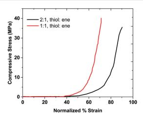
Fig. 6 The compressive stress-strain curves for the hydrogels.
