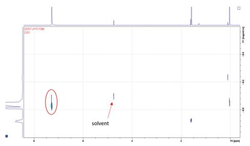
Fig. 3 The DOSY NMR ( $D_2O$ , 400 MHz) spectrum of the 1:1 (thiol:ene) gel after a basic degradation in deuterium oxide. The signal at  $\sim$ 7.5 ppm suggests the presence of only small fragments in the system.
