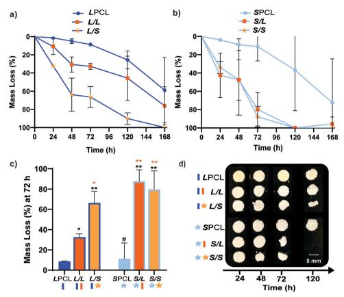
Fig. 3 Gravimetric mass loss over time for base-catalyzed degradation studies (0.2 M NaOH, 37 °C, 60 rpm) for (a) linear-PCL-based and (b) star-PCLbased scaffolds. (c) Mass loss at 72 h was compared for all scaffold compositions; \*p < 0.05, \*\*p < 0.01, #p > 0.05. Note: the black color-coded statistics were compared to LPCL control while orange color-coded statistics were compared to the L/L composition. (d) Representative photos of specimens at different timepoints during degradation study.
