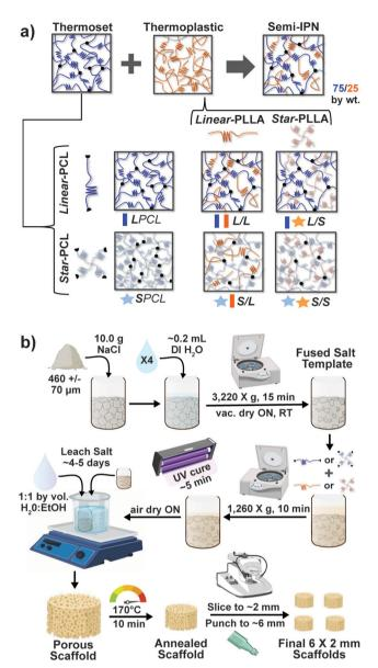
Fig. 1 (a) Four semi-IPN SMP scaffolds were prepared with combinations of linear-PCL-DA or star-PCL-TA and linear-PLLA or star-PLLA (75/25 PCL/PLLA). Two 100% PCL controls were also prepared from linear-PCL-DA or star-PCL-TA. (b) All SMP scaffolds were prepared via solventcasting/particulate leaching (SCPL) whereby a designated solvent-based macromer solution was sequentially cast over a fused salt template, UV-cured, and the template extracted to yield highly interconnected pores.
