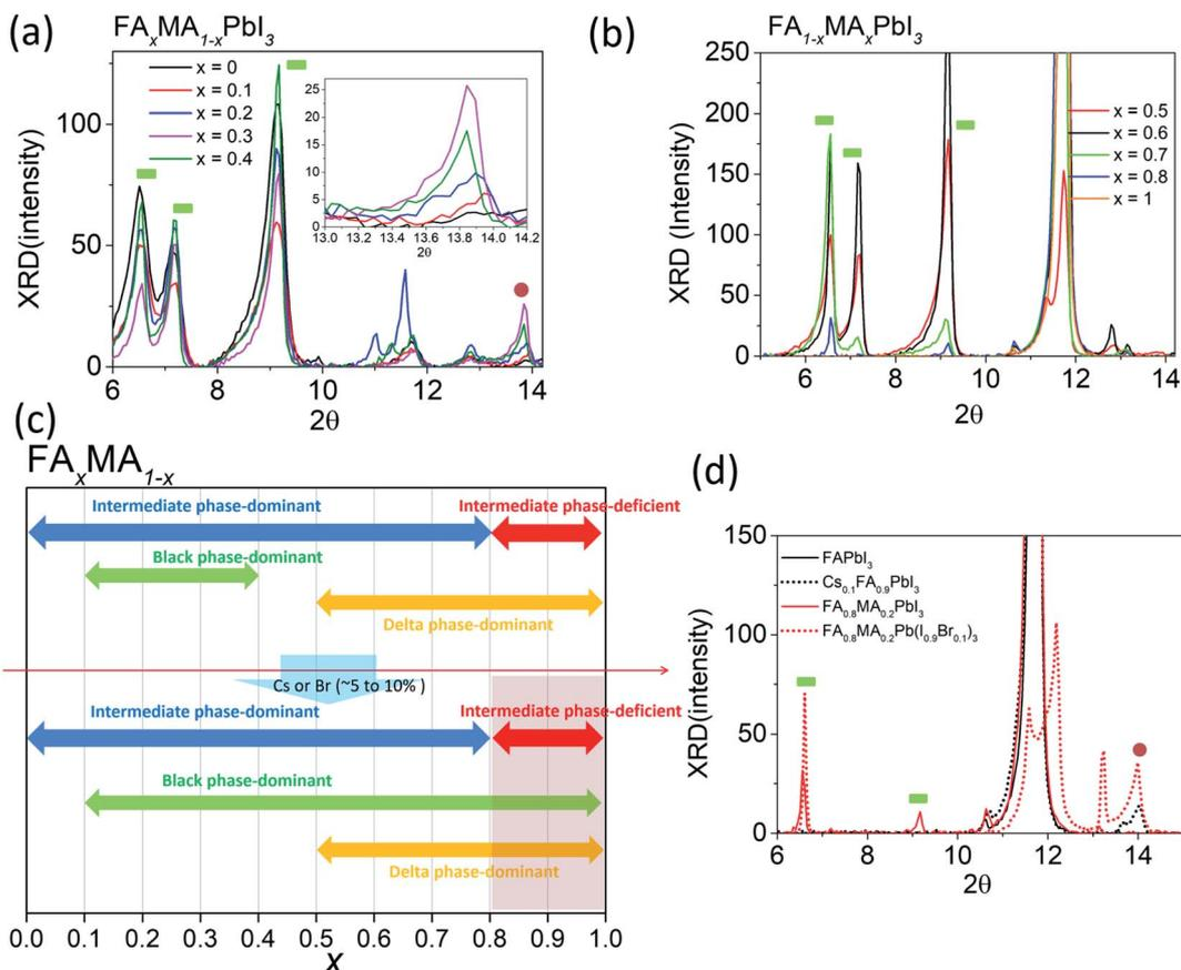
Fig. 4 XRD results for wet films consisting of glass/perovskites ( $\text{FA}_x\text{MA}_{1-x}\text{PbI}_3$ ) at (a)  $x = 0, 0.1, 0.2, 0.3,$  and  $0.4$  and (b)  $x = 0.5, 0.6, 0.7, 0.8,$  and  $1$ . (c) Different phases with respect to  $x$ . (d) XRD results for wet films with/without Cs or Br.
