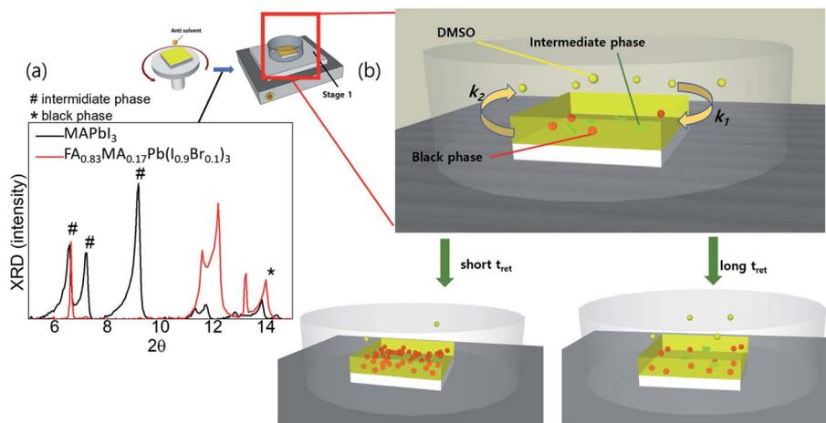
Fig. 2 (a) XRD of wet films (before annealing) for  $\text{MAPbI}_3$  and  $\text{FA}_{0.8}\text{MA}_{0.2}\text{Pb}(\text{I}_{0.9}\text{Br}_{0.1})_3$ ; (b) illustrations of  $t_{\text{ret}}$ -sensitive films at stage 1.
