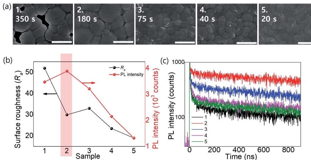
Fig. 5 (a) SEM images, (b)  $R_a$  and PL intensity values, and (c) TRPLs of perovskite films of  $\text{Rb}_{0.03}\text{Cs}_{0.05}(\text{FA}_{0.83}\text{MA}_{0.17})_{0.92}\text{Pb}(\text{I}_{0.83}\text{Br}_{0.17})_3$  with different  $t_{\text{evap}}$  values (20–350 s).
