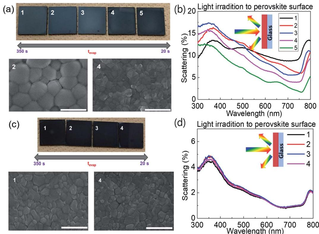
Fig. 1 (a and c) SEM images and (b and d) light-scattering spectra for (a and b) FA<sub>0.8</sub>MA<sub>0.2</sub>Pb(I<sub>0.9</sub>Br<sub>0.1</sub>)<sub>3</sub> and (c and d) MAPbI<sub>3</sub> on glass with different  $t_{\text{evap}}$  values.
