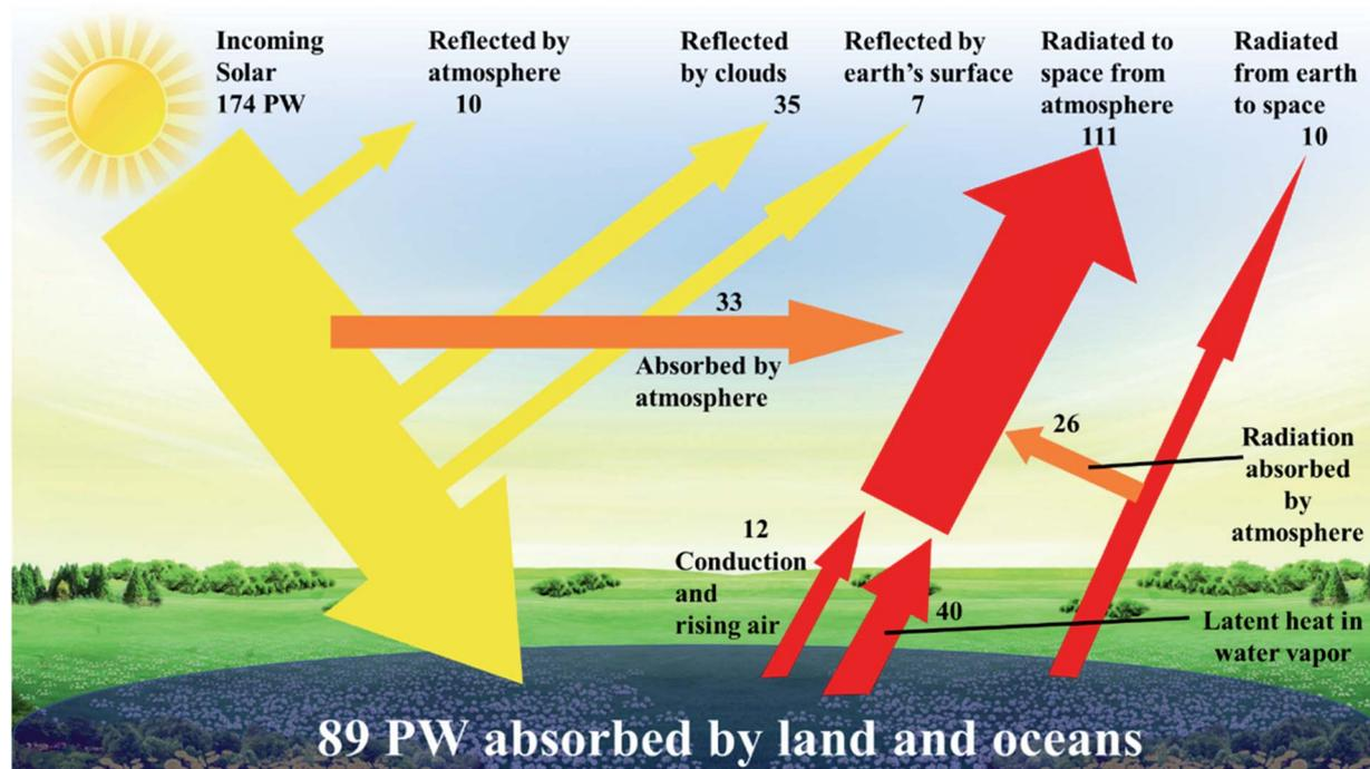
Fig. 1 Incoming solar power distribution is reflected and absorbed in many ways.<sup>5</sup>
