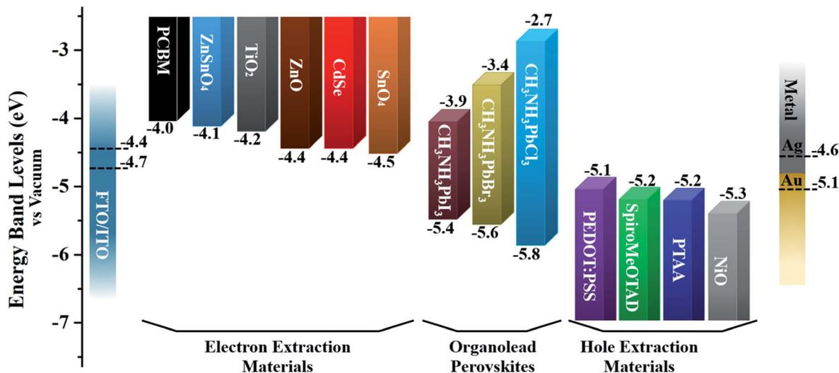
Fig. 5 The band energy level diagram for commonly utilized charge-extraction layer materials and CH<sub>3</sub>NH<sub>3</sub>PbX<sub>3</sub> perovskites. Note: the dotted lines represent the work functions of various electrodes.
