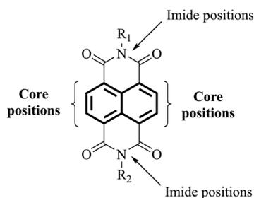
Fig. 7 Structure of naphthalene diimide (NDI) core.
