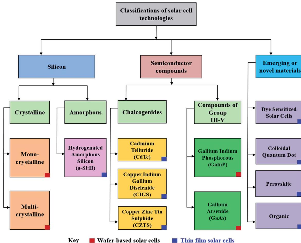
Fig. 2 Alternative classification of solar cells based on the primary light-absorbing material within the device.<sup>27</sup>
