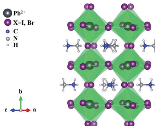
Fig. 3 Structure of a typical perovskite  $ABX_3$  crystal structure where A and B are cations of different sizes, e.g.  $CH_3NH_3^+$  and  $Pb^{2+}$ , and X is a monovalent anion, e.g.  $I^-$  or  $Cl^-$  or  $Br^-$ .
