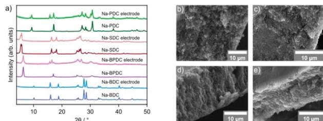
Fig. 4 Characterisation of electrode composites prior to electrochemical cycling experiments. PXRD patterns (normalised) of mechanochemically synthesised sodium carboxylates and the respective electrodes (a) and SEM images of electrodes made with (b) Na-BDC, (c) Na-BPDC, (d) Na-SDC, and (e) Na-PDC.
