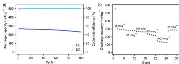
Fig. 5 (a) Galvanostatic cycling performance for Na-BDC at  $100 \text{ mA g}^{-1}$  cycled between  $0.01\text{--}2.5 \text{ V}$ . (b) Rate performance for Na-BDC, cycled 5 times at each current density.
