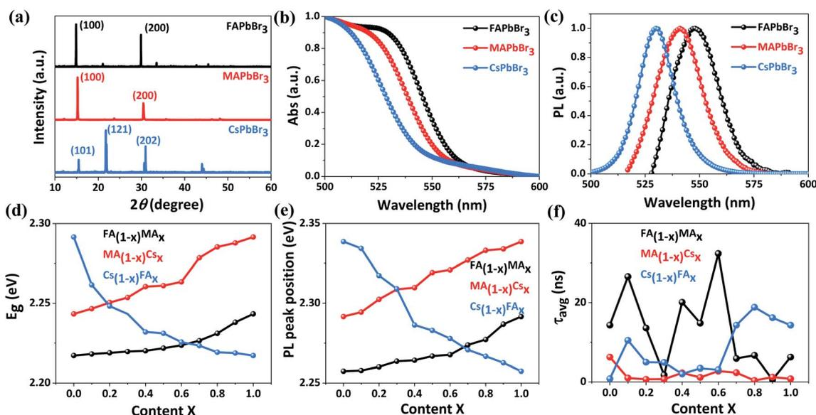
Fig. 4 XRD patterns (a), absorbance spectra (b) and PL spectra (c) of inkjet-printed FAPbBr<sub>3</sub>, MAPbBr<sub>3</sub> and CsPbBr<sub>3</sub> thin films. Bandgaps (d), PL peak positions (e) and average PL lifetimes ( $\tau_{\text{avg}}$ ) (f) of inkjet-printed FA<sub>1-x</sub>MA<sub>x</sub>PbBr<sub>3</sub>, MA<sub>1-x</sub>Cs<sub>x</sub>PbBr<sub>3</sub> and Cs<sub>1-x</sub>FA<sub>x</sub>PbBr<sub>3</sub> films as a function of  $x$ .
