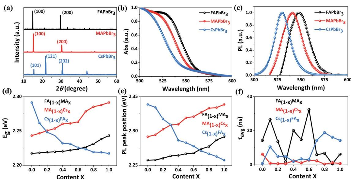
Fig. 4 XRD patterns (a), absorbance spectra (b) and PL spectra (c) of inkjet-printed FAPbBr<sub>3</sub>, MAPbBr<sub>3</sub> and CsPbBr<sub>3</sub> thin films. Bandgaps (d), PL peak positions (e) and average PL lifetimes ( $\tau_{\text{avg}}$ ) (f) of inkjet-printed FA<sub>1-x</sub>MA<sub>x</sub>PbBr<sub>3</sub>, MA<sub>1-x</sub>Cs<sub>x</sub>PbBr<sub>3</sub> and Cs<sub>1-x</sub>FA<sub>x</sub>PbBr<sub>3</sub> films as a function of  $x$ .
