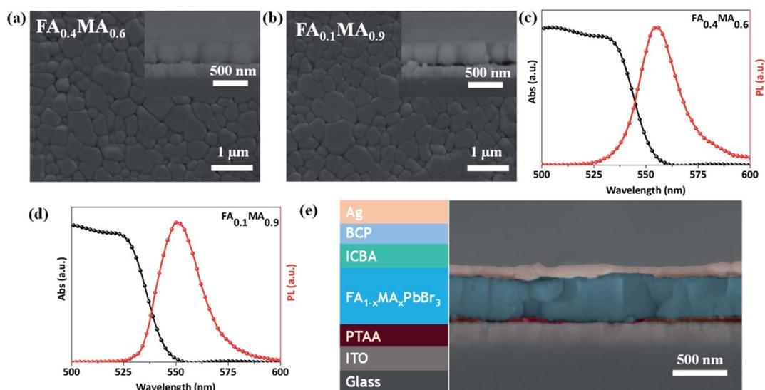
Fig. 5 Top-view and cross-sectional SEM images of spin-coated FA<sub>0.4</sub>MA<sub>0.6</sub> (a) and FA<sub>0.1</sub>MA<sub>0.9</sub> (b) films, respectively. Steady-state PL spectra and absorbance spectra of spin-coated FA<sub>0.4</sub>MA<sub>0.6</sub> (c) and FA<sub>0.1</sub>MA<sub>0.9</sub> (d) films, respectively. (e) Cross-sectional SEM image of a typical cell with a structure of ITO/PTAA/perovskite/ICBA/BCP/Ag.
