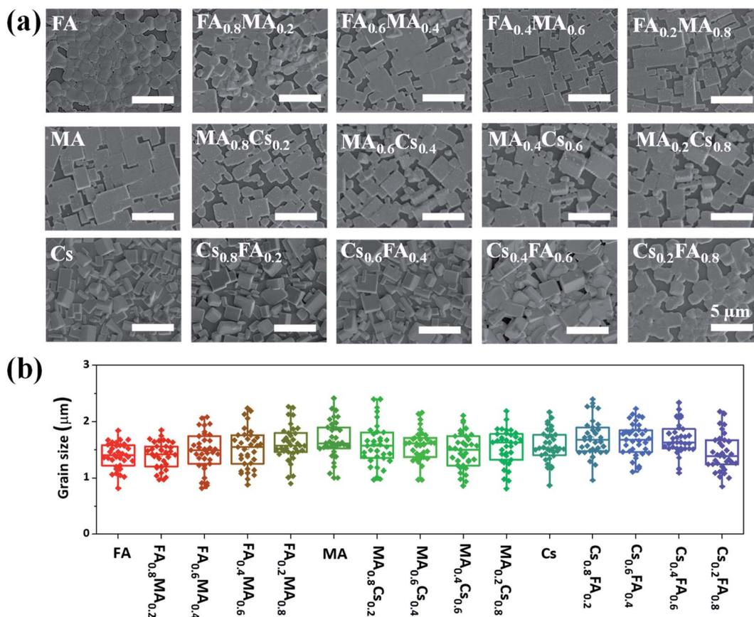
Fig. 3 (a) Top-view SEM images of inkjet-printed  $FA_{1-x}MA_xPbBr_3$ ,  $MA_{1-x}Cs_xPbBr_3$  and  $Cs_{1-x}FA_xPbBr_3$  thin films with  $x = 0, 0.2, 0.4, 0.6$ , and  $0.8$ , respectively. (b) Statistical distributions of the grain size of these inkjet-printed films.
