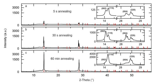
Fig. 2 XRD data of MAPbl<sub>3</sub> samples that were thermally annealed for (a) 5 s, (b) 30 s and (c) 60 min. After 5 s of annealing, no more precursor residues were found. The texture gradually changes from non-uniform with local (002) and (110) orientation to a prevailing (110) texture.
