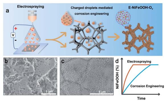
Fig. 1 (a) Schematic illustration of the reaction process of E-NiFeOOH composites *via* electrospraying. (b) SEM images of I-NiFeOOH-20 min. (c) SEM images of E-NiFeOOH-20 min. (d) The content (%) of NiFeOOH changes over time in different systems: electrospraying and corrosion engineering.
