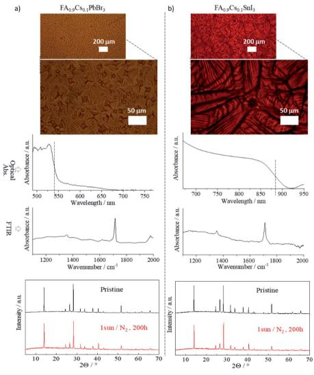
Fig. 5 Optical image, absorption spectra, FTIR spectra and XRD pattern for (a) FA<sub>0.9</sub>Cs<sub>0.1</sub>PbBr<sub>3</sub> and (b) FA<sub>0.9</sub>Cs<sub>0.1</sub>SnI<sub>3</sub> perovskite thin films, annealed at 1.4 s  $t_{\rm f}$
