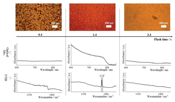
Fig. 1 Film evolution during annealing. Optical images are measured in transmission mode. Optical absorption spectra, and FTIR measurement were performed on a single spot for  $FA_{0.85}MA_{0.1}Cs_{0.05}Pbl_3$  perovskite composition and three flash times.
