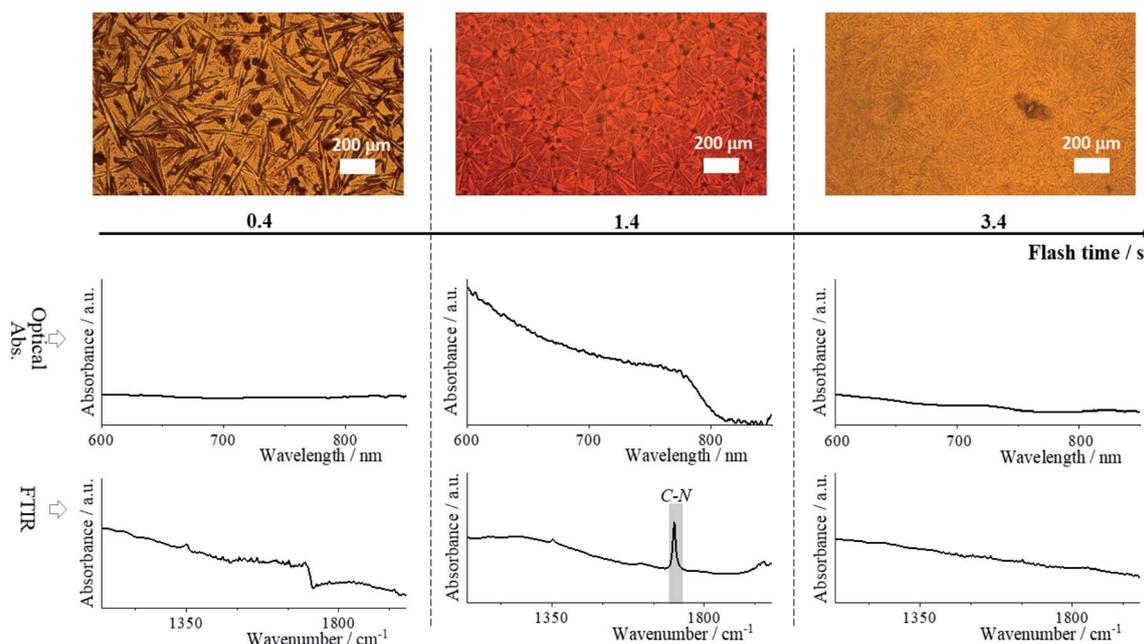
Fig. 1 Film evolution during annealing. Optical images are measured in transmission mode. Optical absorption spectra, and FTIR measurement were performed on a single spot for  $\text{FA}_{0.85}\text{MA}_{0.1}\text{Cs}_{0.05}\text{PbI}_3$  perovskite composition and three flash times.
