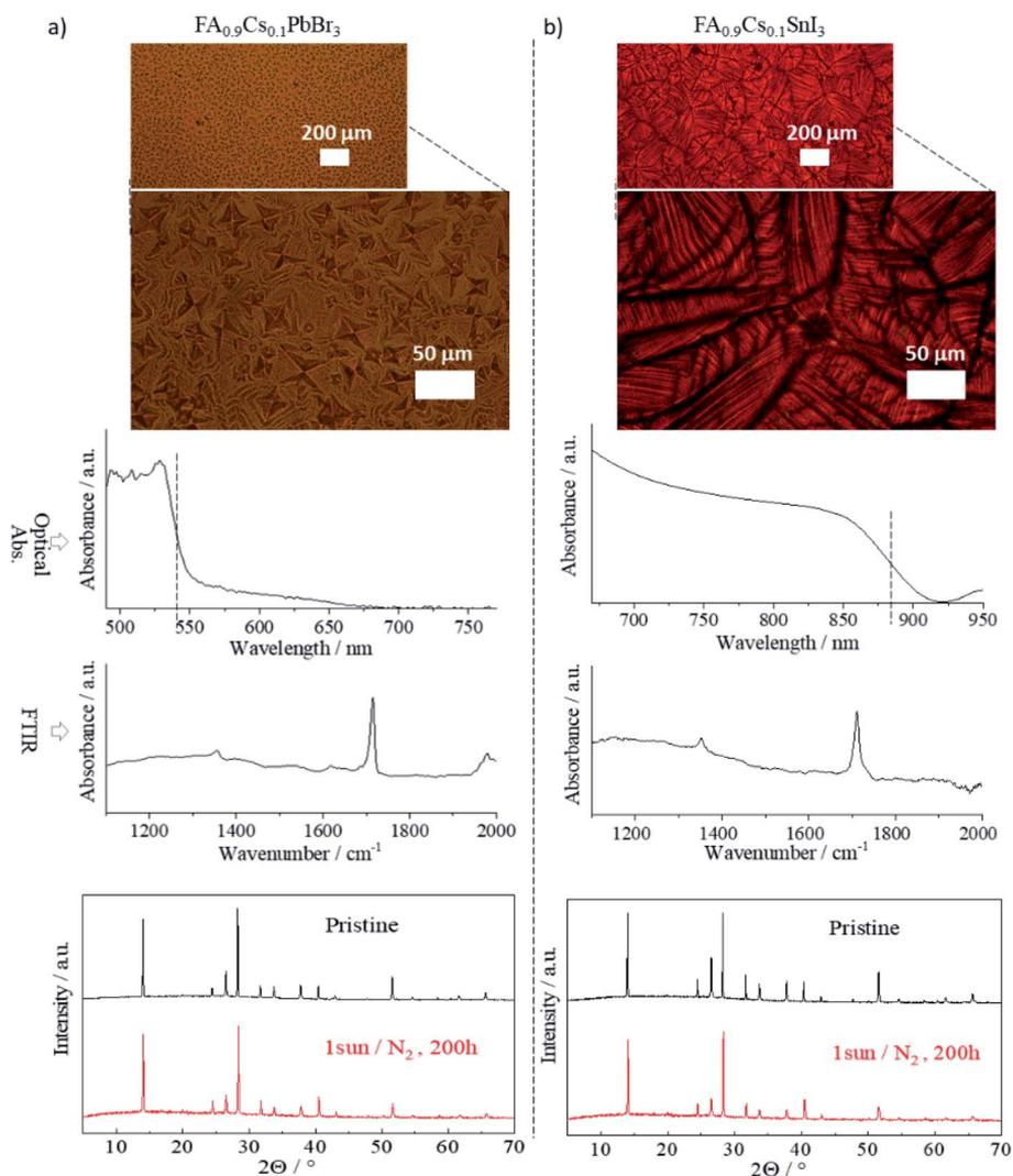
Fig. 5 Optical image, absorption spectra, FTIR spectra and XRD pattern for (a)  $\text{FA}_{0.9}\text{Cs}_{0.1}\text{PbBr}_3$  and (b)  $\text{FA}_{0.9}\text{Cs}_{0.1}\text{SnI}_3$  perovskite thin films, annealed at 1.4 s  $t_f$ .
