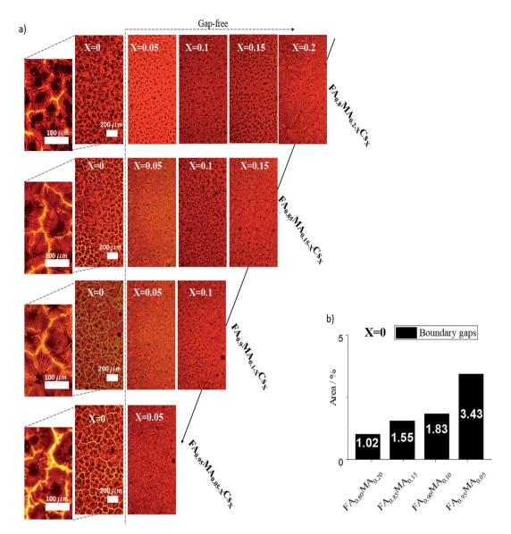
(a) Optical images of the fourteen selected perovskite films. (b) Area percent of gaps with respect to grain domains for the Cs-free films.
