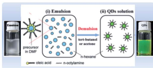
Fig. 10 Illustration of the emulsion synthesis method and photographs of the  $MAPbBr_3$  emulsion and the resultant colloidal solution upon addition of the demulsifier. Modified with permission from ref. 162.
