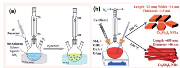
Fig. 6 (a) Schematic illustrating the HI method (b) Scheme presenting the HI synthesis of Cs<sub>3</sub>Sb<sub>2</sub>I<sub>9</sub> NPLs and NRs at different temperatures using octanoic acid (OnA) and oleylamine (OAm) ligands in 1-octadecene (ODE). Panels (a) and (b) are taken with permission from ref. 14 and 134, respectively.
