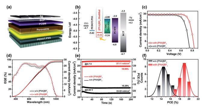
Fig. 4 (a) The device structure of mixed Sn-Pb perovskite PSCs treated by [PNA]BF4 ionic salts; (b) energy-level diagram of each layer related devices; (c) J-V curves of champion PSCs under AM 1.5G 100 mW cm<sup>-2</sup> illumination; (d) EQE spectra of corresponding PSCs; (e) steady-state  $J_{sc}$ and corresponding efficiencies of champion devices (at 0.70 V for the PSC with [PNA]BF4, at 0.65 V for the PSC without [PNA]BF4); (f) performance distribution diagram for 20 devices in one bath.
