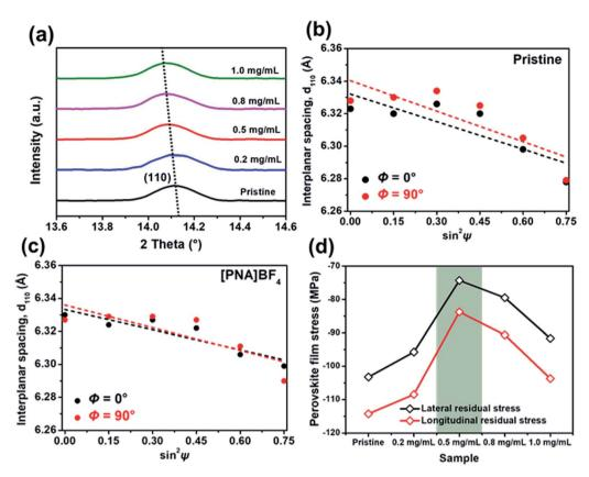
Fig. 3 (a) XRD spectra of magnified (110) lattice plane diffraction peaks for perovskite films grown on PEDOT:PSS and different concentrations of the [PNA]BF<sub>4</sub> layer; XRD  $d_{110}$  versus  $\sin^2 \psi$  plots for perovskite film grown on (b) PEDOT:PSS and (c) [PNA]BF<sub>4</sub> layer (5 mg mL<sup>-1</sup>); (d) lateral and longitude residual stress (or strain) of perovskite films based on PEDOT:PSS and different concentration [PNA]BF4 layer.
