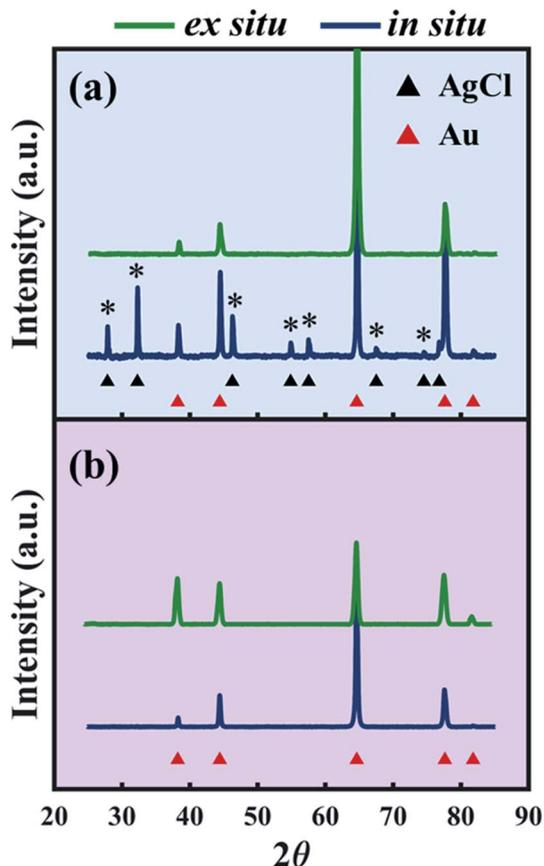
Fig. 4 (a) XRD patterns after dealloying in 1 M  $\text{HClO}_4$  in small volumes (*in situ*, blue) and in large volumes (*ex situ*, green). Asterisks mark the AgCl peaks (PDF # 31-1238) formed during *in situ* dealloying. (b) XRD patterns after dealloying in 1 M  $\text{HNO}_3$  in small volumes (*in situ*, blue) and in large volumes (*ex situ*, green).
