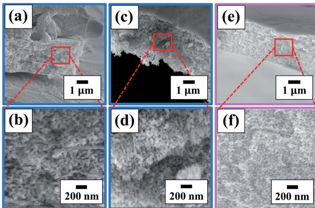
Fig. 5 SEM images of *in situ* dealloyed NP-Au. (a and b) NP-Au dealloyed in  $\text{HClO}_4$ , with large AgCl particles on the top surface of the film. (c and d) NP-Au dealloyed in  $\text{HClO}_4$  and washed in 17 M  $\text{NH}_3$  to remove residual AgCl particles. (e and f) NP-Au dealloyed in  $\text{HNO}_3$ .
