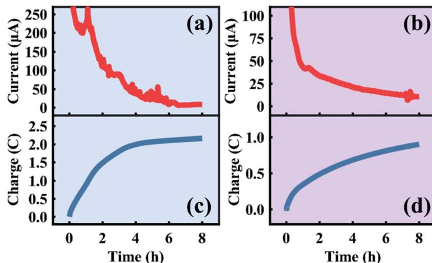
Fig. 2 Current and charge transferred during the first eight hours of the *in situ* sample dealloyed in HClO<sub>4</sub> (a and c) and HNO<sub>3</sub> (b and d).
