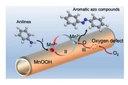
Scheme 1 The proposed catalytic process for oxidative coupling of anilines using NT-MnOOH.
