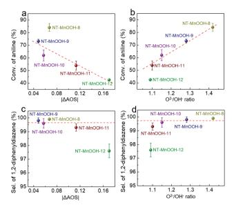
Fig. 4 The conversion of aniline as functions of (a) surface Mn<sup>3+</sup> fraction and (b) surface oxygen defects. The selectivity of 1,2-diphenyldiazene as functions of the (c) surface Mn3+ fraction and (d) surface oxygen defects. Reaction conditions: aniline (0.5 mmol), catalysts (20 mg), toluene (2 mL), 0.5 MPa O<sub>2</sub>, 60 °C and 8 h.
