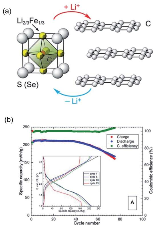
Fig. 6 Anti-perovskite cathode materials. (a) Schematic representation of a graphite|Li<sub>2</sub>FeSO battery cell. Reproduced with permission from ref. 100 Copyright (2017) American Chemical Society. (b) Specific capacity, coulombic efficiency and inset voltage profiles of a Li<sub>2</sub>-FeSO|Li cell cycled at a 1C rate. Reproduced with permission from ref. 171 Copyright (2021) Frontiers.
