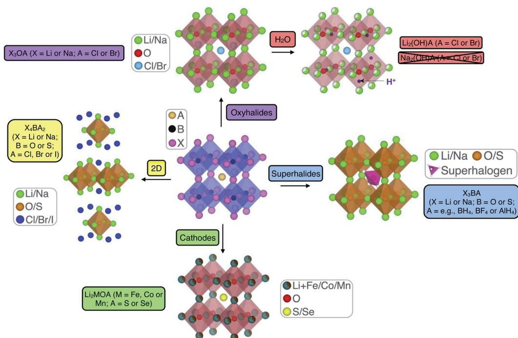
Fig. 1 Schematic highlighting the structural and compositional versatility of anti-perovskite battery materials.
