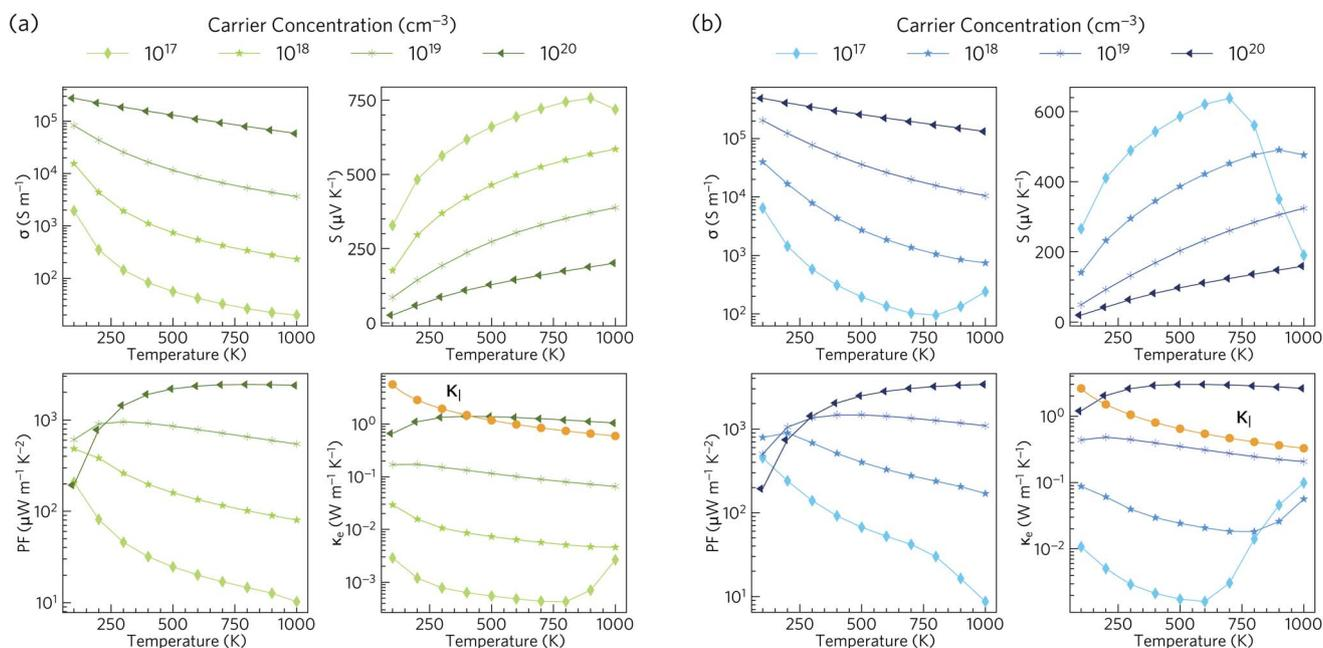
Fig. 6 Calculated electronic transport properties as a function of temperature for p-type  $\text{Ca}_4\text{Sb}_2\text{O}$  (a) and  $\text{Ca}_4\text{Bi}_2\text{O}$  (b) at four different carrier concentrations: electrical conductivity ( $\sigma$ ), Seebeck coefficient ( $S$ ), power factor (PF) and electronic thermal conductivity ( $\kappa_e$ ). The lattice thermal conductivity ( $\kappa_l$ ; see Section 3.5) is indicated on the  $\kappa_e$  plots with orange lines for comparison.
