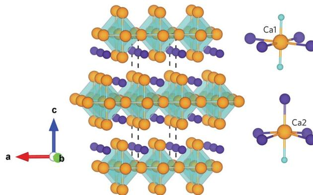
Fig. 1 Crystal structure of Ca<sub>4</sub>Sb<sub>2</sub>O and Ca<sub>4</sub>Bi<sub>2</sub>O showing the O-centred Ca octahedra stacked along the crystallographic *c* axis. The insets show the coordination polyhedra around the two distinct Ca atoms. The atoms are coloured as follows: Ca – orange, O – cyan, Sb/Bi – purple. The images were generated using the VESTA software.<sup>33</sup>
