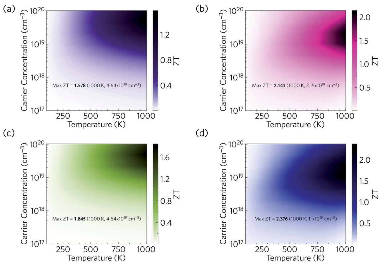
Fig. 17 Predicted thermoelectric figure of merit  $ZT$  of p-type doped  $\text{Ca}_4\text{Sb}_2\text{O}$  (a/c) and  $\text{Ca}_4\text{Bi}_2\text{O}$  (b/d) as a function of temperature and carrier concentration. (a) and (b) show predictions based on the lattice thermal conductivity of bulk single crystals, while (c) and (d) show the enhanced  $ZT$  obtained by nanostructuring down to a grain size of 20 nm to limit the  $\kappa_1$ .
