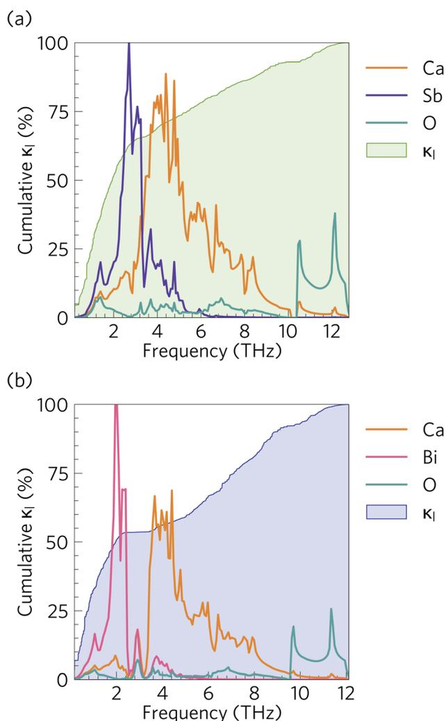
Fig. 10 Cumulative % lattice thermal conductivity of (a)  $\text{Ca}_4\text{Sb}_2\text{O}$  and (b)  $\text{Ca}_4\text{Bi}_2\text{O}$  as a function of frequency at  $T = 300$  K (green/blue shaded areas) overlaid against the phonon density of states projected onto Ca (orange), Sb (purple), Bi (pink) and O (cyan) atoms.
