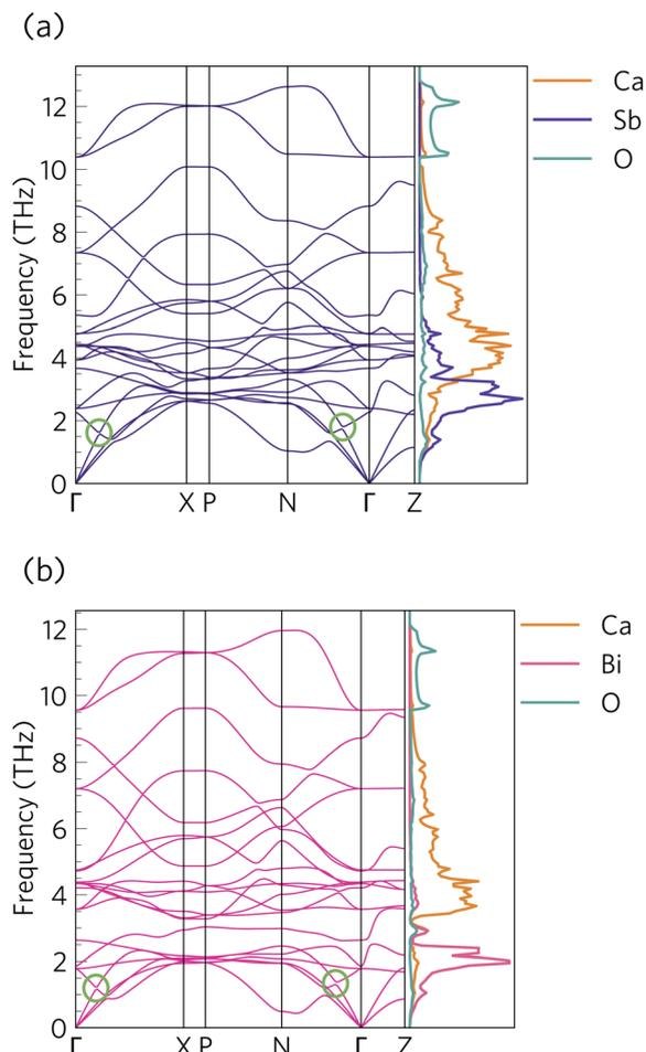
Fig. 8 Harmonic phonon dispersion and atom-projected density of states (pDoS) curves for  $\text{Ca}_4\text{Sb}_2\text{O}$  (a) and  $\text{Ca}_4\text{Bi}_2\text{O}$  (b). Projections of the DoS onto Ca, Sb, Bi and O atoms are displayed in orange, purple, pink, and cyan, respectively. Avoided crossings between acoustic and optic modes are marked by green circles in the dispersions.
