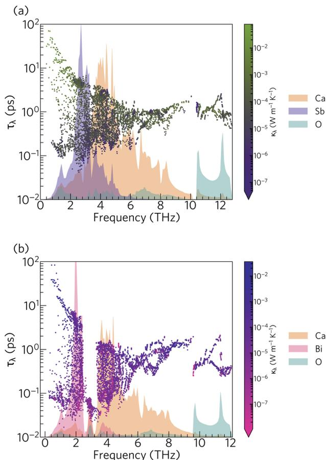
Fig. 13 Frequency spectra of the phonon lifetimes  $\tau_\lambda$  in  $\text{Ca}_4\text{Sb}_2\text{O}$  (a) and  $\text{Ca}_4\text{Bi}_2\text{O}$  (b) at  $T = 300$  K, overlaid against the phonon density of states projected onto the Ca (orange), Sb (purple), Bi (pink) and O (cyan) atoms.
