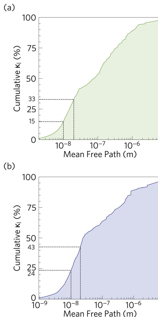
Fig. 11 Cumulative % lattice thermal conductivity of  $\text{Ca}_4\text{Sb}_2\text{O}$  (a) and  $\text{Ca}_4\text{Bi}_2\text{O}$  (b) at  $T = 300$  K as a function of the phonon mean free paths. The percentage of the lattice thermal conductivity from phonons with mean free paths less than 20 nm and 10 nm are indicated by dashed black lines.
