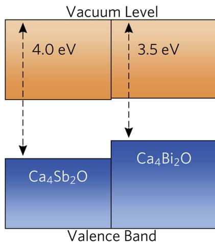
Fig. 5 Band alignment of  $\text{Ca}_4\text{Sb}_2\text{O}$  and  $\text{Ca}_4\text{Bi}_2\text{O}$  using slab models, with energies calculated relative to the O 1s core levels. The valence and conduction bands are coloured in blue and orange respectively.
