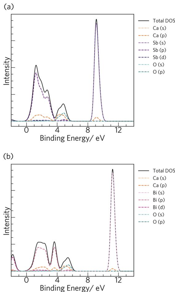
**Fig. 4** Simulated X-ray photoelectron spectra (0.3–2 keV) for  $\text{Ca}_4\text{Sb}_2\text{O}$  (a) and  $\text{Ca}_4\text{Bi}_2\text{O}$  (b), obtained from electronic density-of-states calculations performed at the HSE06 + SOC level of theory.
