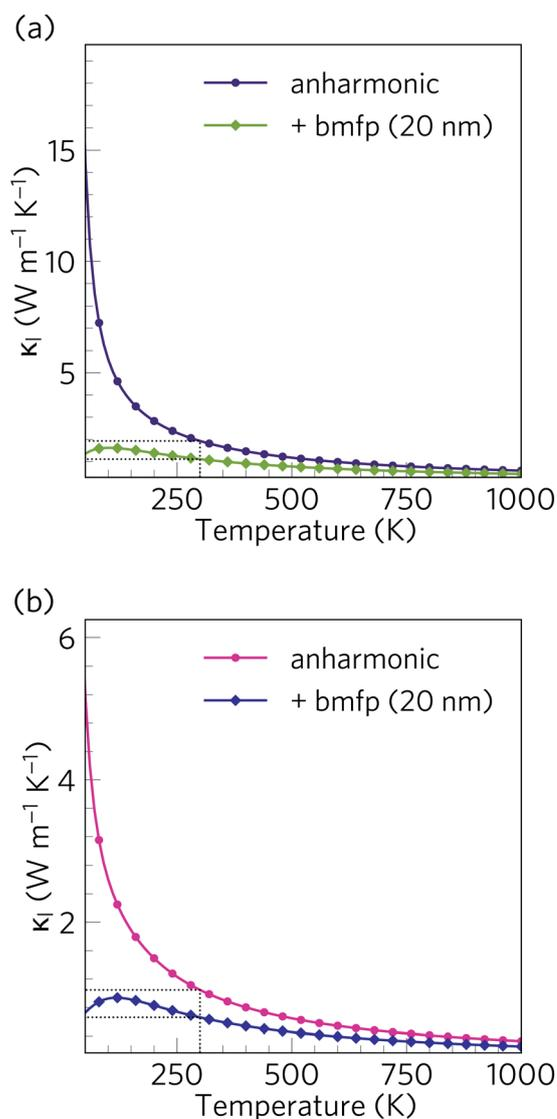
Fig. 16 Isotropically averaged lattice thermal conductivity  $\kappa_l$  of  $\text{Ca}_4\text{Sb}_2\text{O}$  (a) and  $\text{Ca}_4\text{Bi}_2\text{O}$  (b) as a function of temperature without (circles) and with (diamonds) a boundary-scattering model applied to mimic a crystal grain size of 20 nm.
