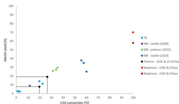
Fig. 1 Comparison of CO<sub>2</sub> conversion and methanol yield for membrane reactors (MR) with results for traditional reactors (TR). TR: light blue.<sup>9,11</sup> MR (2004): purple.<sup>9</sup> MR (2015): green.<sup>10</sup> MR (2020): dark blue.<sup>8</sup> Thermodynamic equilibrium at 250 °C and 25–50 bar: black. Theoretical maximum at 230–250 °C and 50 bar: red.
