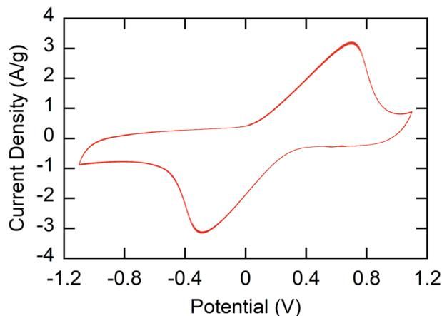
Fig. 2 Cyclic voltammetry of the P1-CNT/Ti electrode's final 10 cycles (from over 100 cycles) in the presence of 100 mM NaClO<sub>4</sub>. The potential range chosen was from –1.1 to 1.1 V with a scan rate of 50 mV s<sup>-1</sup>.
