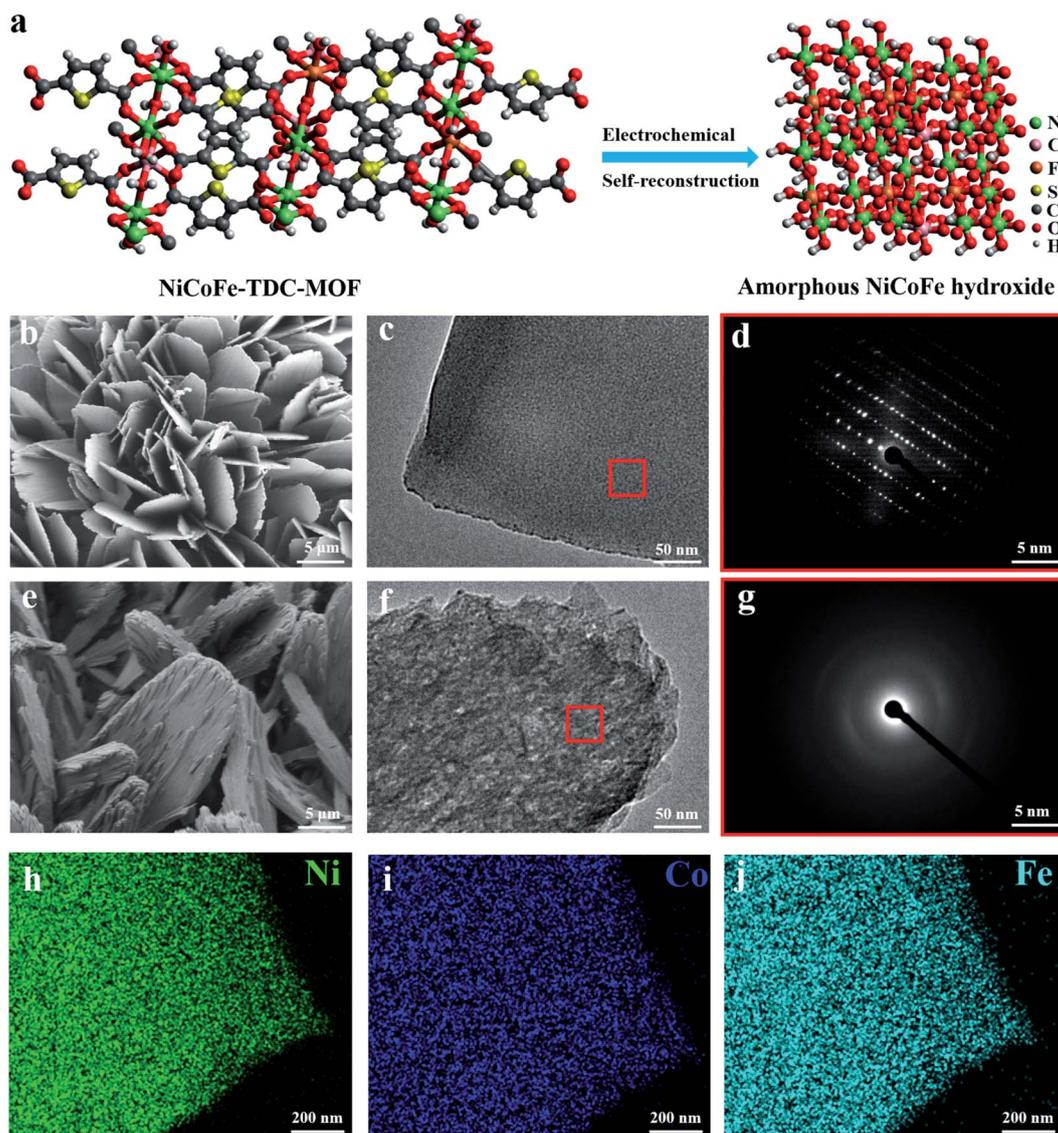
**Fig. 1** Structural characterization of NiCoFe-TDC and NiCoFe-TDC-AC. (a) Schematic diagram for the self-reconstruction result of the NiCoFe-TDC pre-catalyst under electro-oxidation conditions. (b) SEM image, (c) TEM images, and (d) the corresponding FFT spectrum of NiCoFe-TDC. (e) SEM image, (f) TEM images, and (g) the corresponding FFT spectrum of NiCoFe-TDC-AC. STEM EDX chemical maps for (h) Ni, (i) Co, and (j) Fe of a representative NiCoFe-TDC-AC nanosheet.
