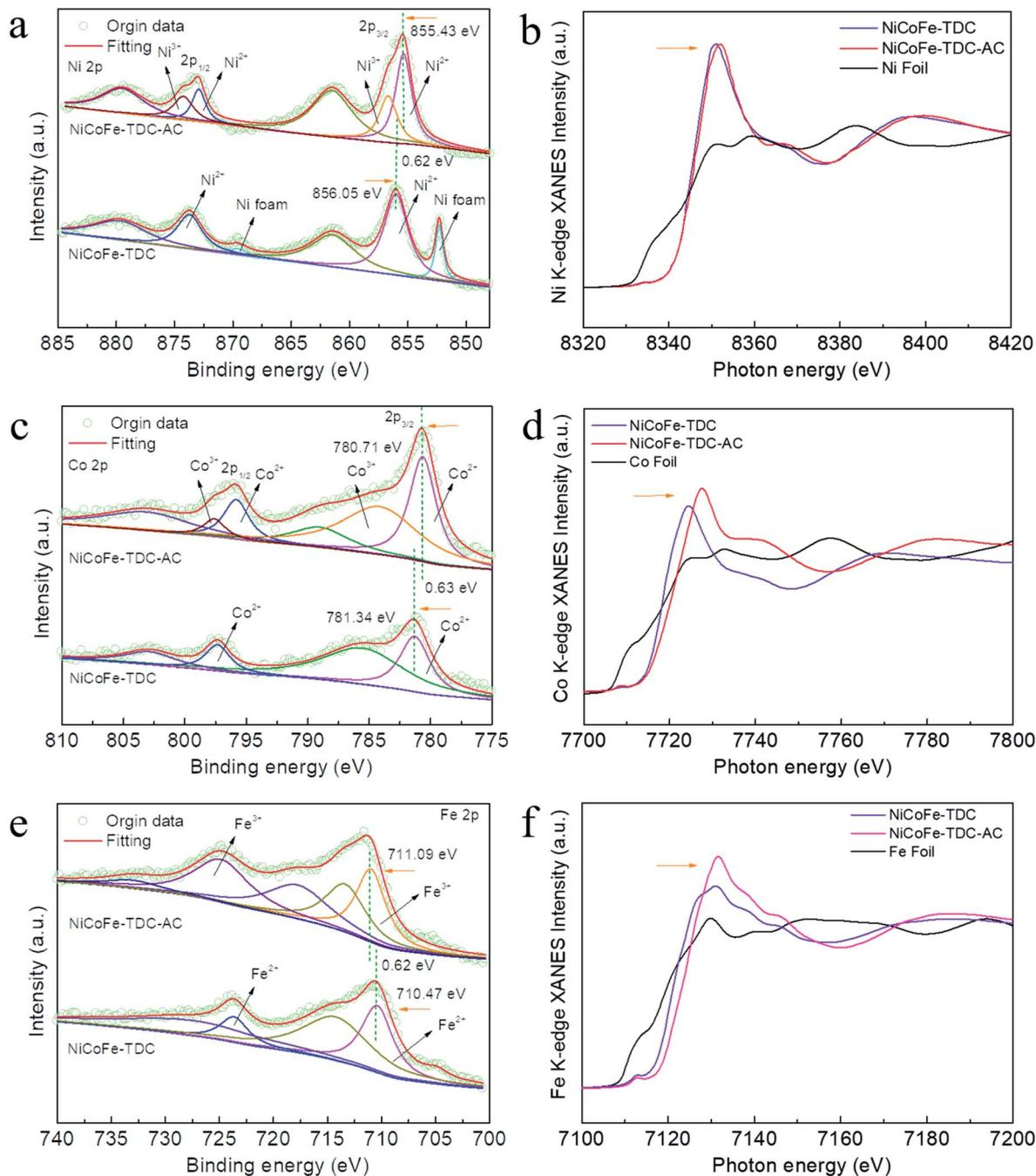
**Fig. 3** Electronic structure characterization and mechanistic investigations of NiCoFe-TDC and NiCoFe-TDC-AC. (a) High resolution Ni 2p, (b) normalized Ni K-edge XANES spectra, (c) high resolution Co 2p, (d) normalized Co K-edge XANES spectra, (e) high resolution Fe 2p, and (f) normalized Fe K-edge XANES spectra.
